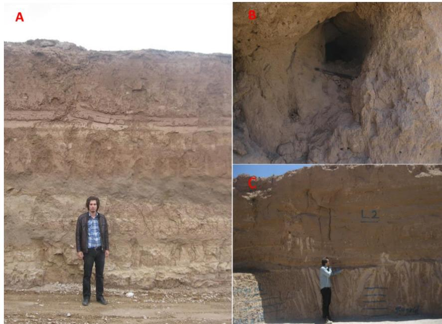
Fig. 15. A) Fine-grained clay and sand sequence B) Soils with solvable holes and collapsible C) Windy sands with high collapsibility property.
