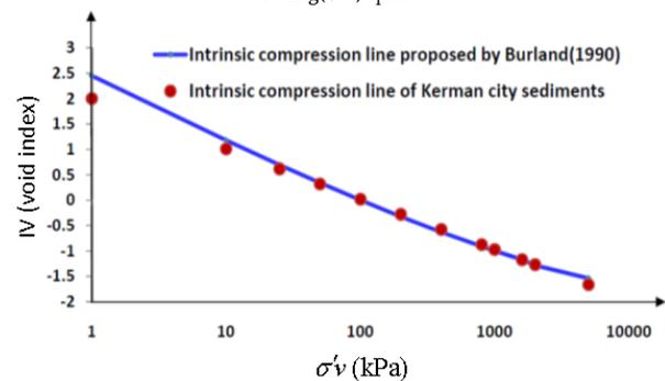
Fig. 4. Comparison of Burland (1990) intrinsic compression line to the Kerman city sediments-ICL.
