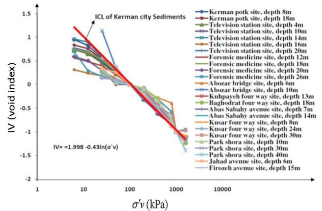
Fig. 3. Extraction of intrinsic compression curves of the Kerman city sediments in Iv-Log( $\sigma'_v$ ) space.
