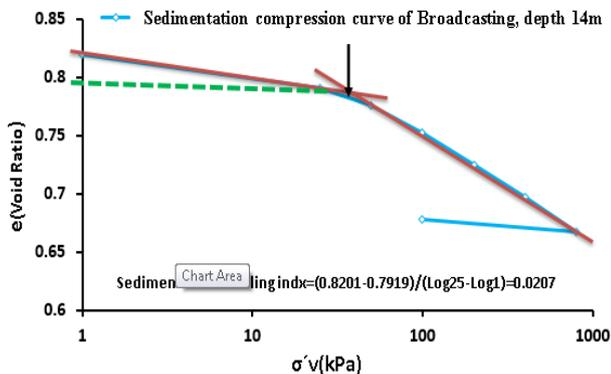
**Fig. 12.** Sedimentation Swelling Index of the Broadcasting site, depth 14 m.
