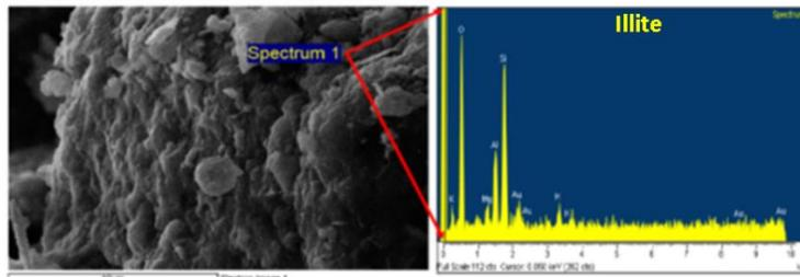
Fig. 6. SEM Photomicrograph and EDX semi-qualitative analysis on sample K9.
