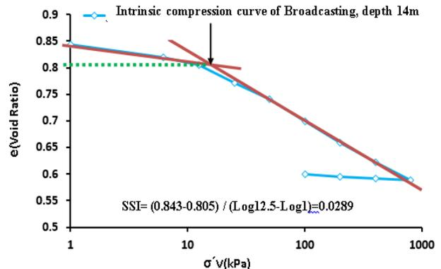
**Fig. 13.** Intrinsic Swelling Index of the Broadcasting site, depth 14 m.
