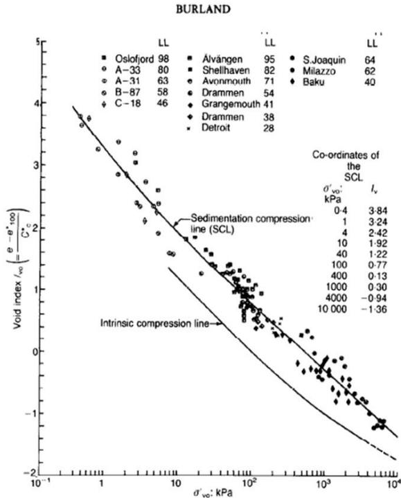
Fig. 5. Relationship between  $I_{v0}$  and  $\log \sigma_v^*$  for many of the normally consolidated clays.
