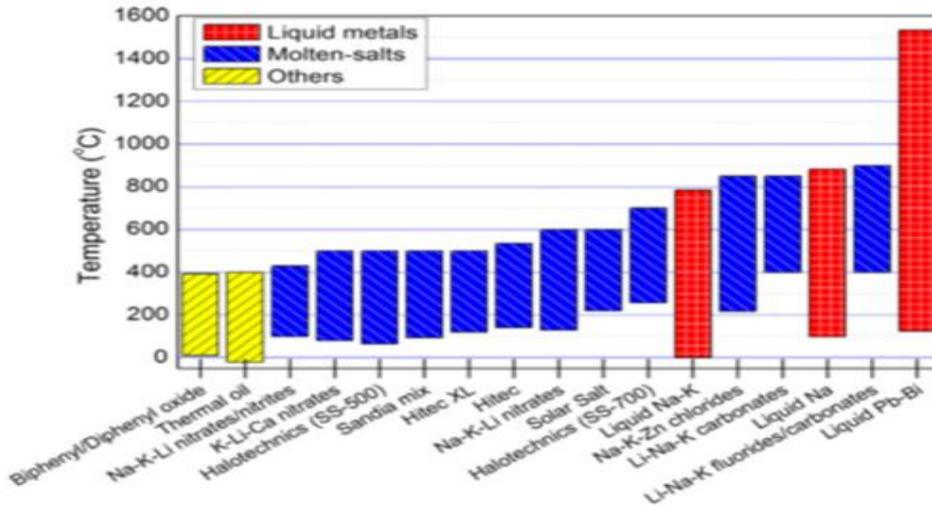
Figure 10. Operating temperature range for various HTFs [5].
