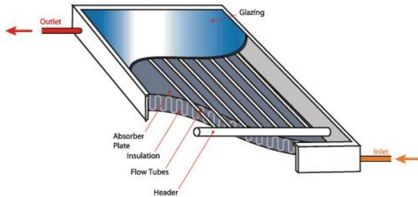
Figure 3. Schematic view of an FPC [6].
