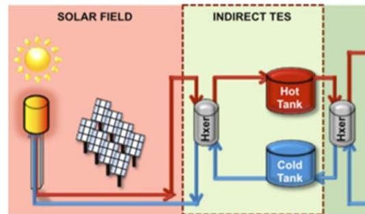
Figure 13. Two-tanks indirect TES system integrated into a CSP plant [21].
