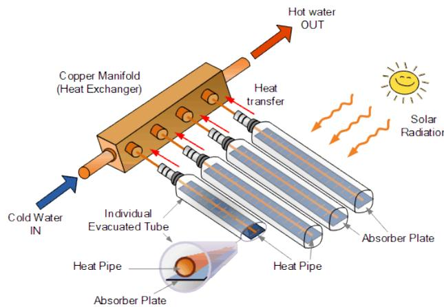
Figure 4. Schematic view of a typical ETC.
