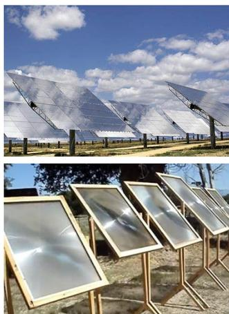
Figure. 2. Solar mirrors (upper) and solar lenses (lower) which both concentrate solar radiation.
