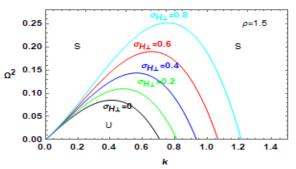
**Figure 3:** Influence of the variation of the vertical magnetic field on the stability diagram for the system of Fig (2). The graph is constructed for  $\Omega^2$  Versus *k*.
