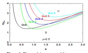
**Figure 1:** The graph is constructed for  $\sigma_{H\perp}$  versus the wavenumber *k* of condition (42). Influence of the angular velocity on the linear stability criteria for variation of  $\Omega$ . The system has  $\rho = 0.5$ .
