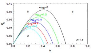
**Figure 4:** As in Fig (3), except that the variation of the vertical magnetic field is replaced by the variation of the tangential field
