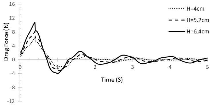
Fig. 23. Impact of water depth on variations of drag force exerted on the cylindrical TLD at 30° angle
