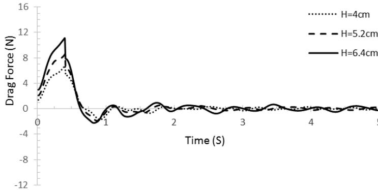
Fig. 24. Impact of water depth on variations of drag force exerted on the cylindrical TLD at 45° angle
