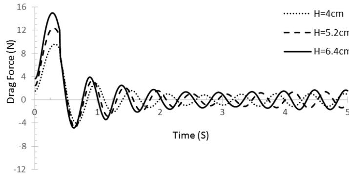
**Fig. 20.** Impact of water depth on variations of drag force exerted on the rectangular TLD at 70° angle
