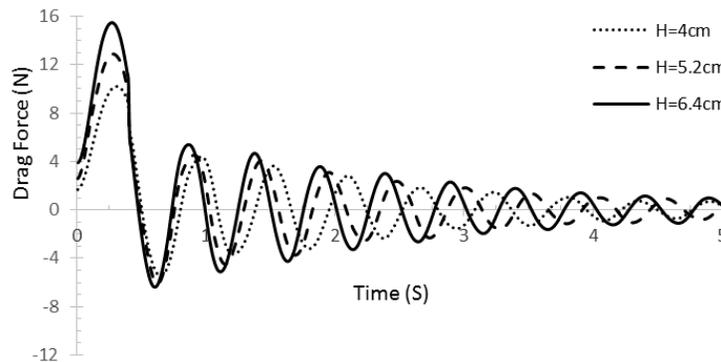
**Fig. 21.** Impact of water depth on variations of drag force exerted on the rectangular TLD at 80° angle
