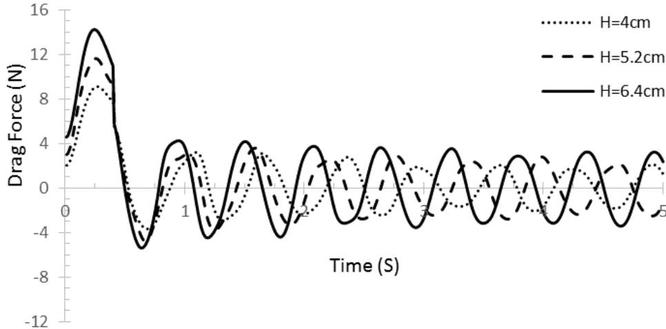
Fig. 26. Impact of water depth on variations of drag force exerted on the cylindrical TLD at 80°angle
