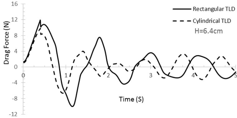
Fig. 12. Variations of drag force exerted on the TLDs at an angle of  $0^\circ$
