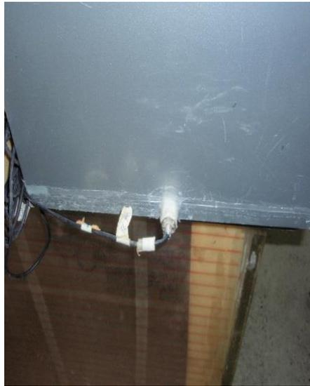
Fig. 10. Installation of the pressure gauges on the bottom of the rectangular TLD
