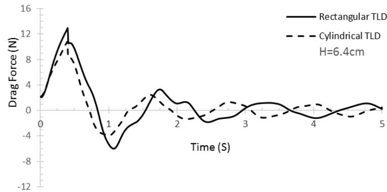
Fig. 13. Variations of drag force exerted on the TLDs at an angle of  $30^\circ$
