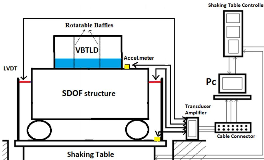
Fig. 4. Schematic view of test set-up and instrumentation
