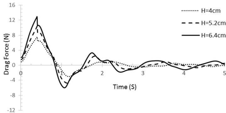
Fig. 18. Impact of water depth on variations of drag force exerted on the rectangular TLD at 30° angle
