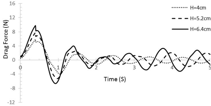
Fig. 22. Impact of water depth on variations of drag force exerted on the cylindrical TLD at 0° angle
