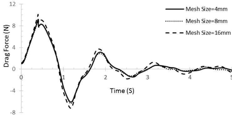
Fig. 2. Comparing drag forces of the rectangular TLD for different Size of the mesh elements
