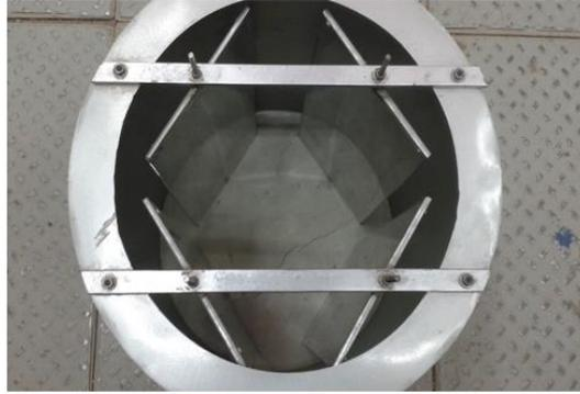
**Fig. 5.** Designed cylindrical TLD with 4 standing rotatable baffles
