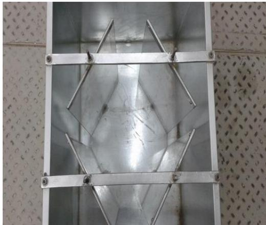
**Fig. 6.** Designed rectangular TLD with 4 standing rotatable baffles
