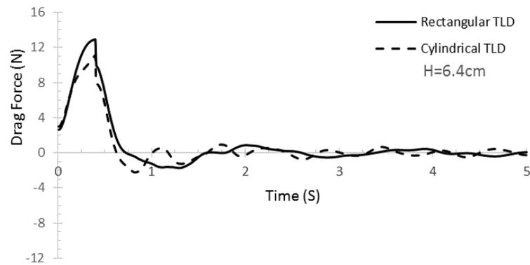
Fig. 14. Variations of drag force exerted on the TLDs at an angle of  $45^\circ$
