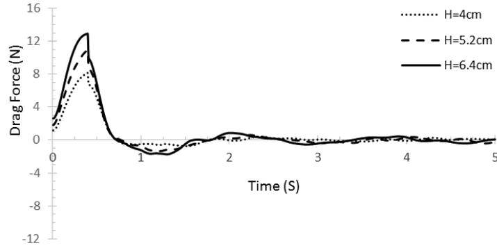
**Fig. 19.** Impact of water depth on variations of drag force exerted on the rectangular TLD at 45° angle
