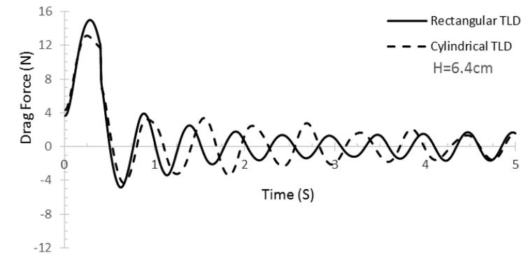
Fig. 15. Variations of drag force exerted on the TLDs at an angle of  $70^\circ$
