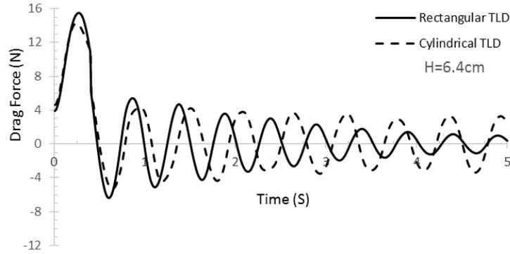
Fig. 16. Variations of drag force exerted on the TLDs at an angle of 80°
