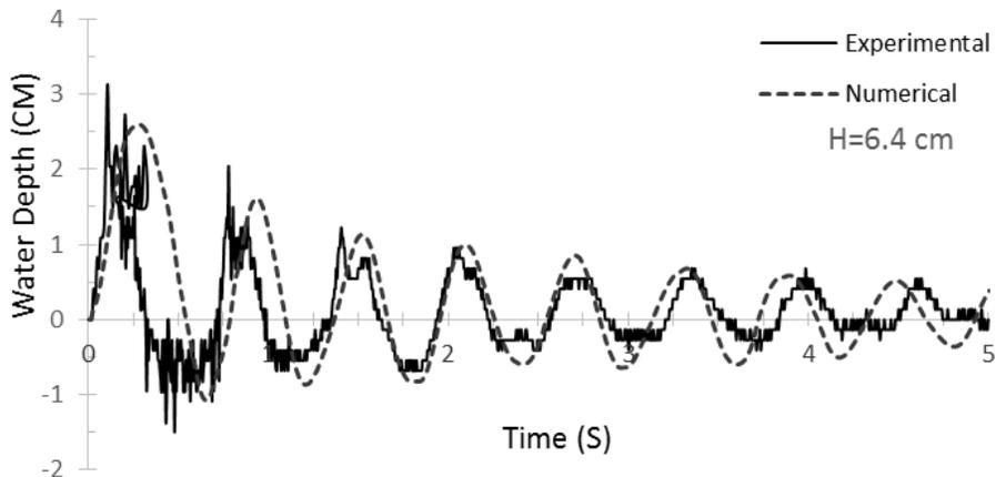
Fig. 11. Comparison of experimental and numerical results on variation of the water level inside the rectangular TLD under pulse excitation
