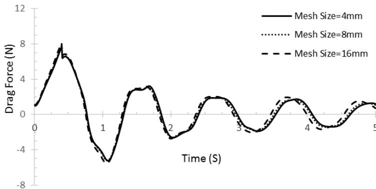
Fig. 3. Comparison drag force of cylindrical TLD for different size of the mesh elements
