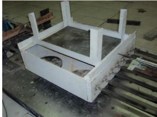
**Fig. 7.** Single Degree-Of-Freedom (SDOF) structure (mass-spring system) used for the test specimen
