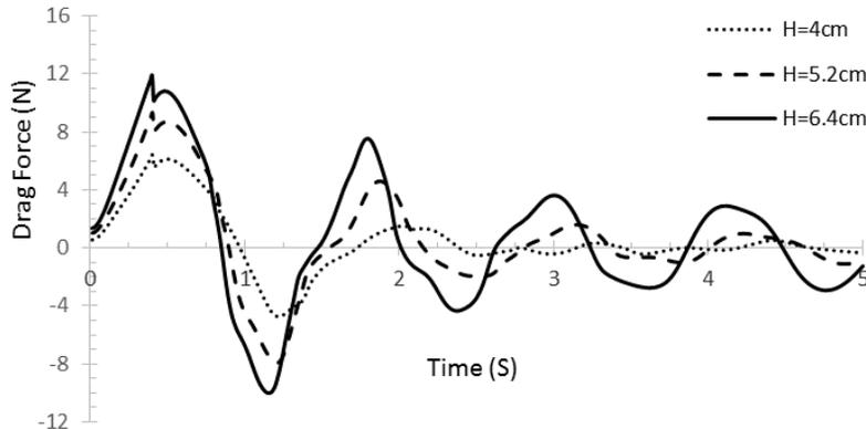
Fig. 17. Impact of water depth on variations of drag force exerted on the rectangular TLD at 0° angle
