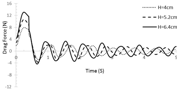
Fig. 25. Impact of water depth on variations of drag force exerted on the cylindrical damper at 70° angle
