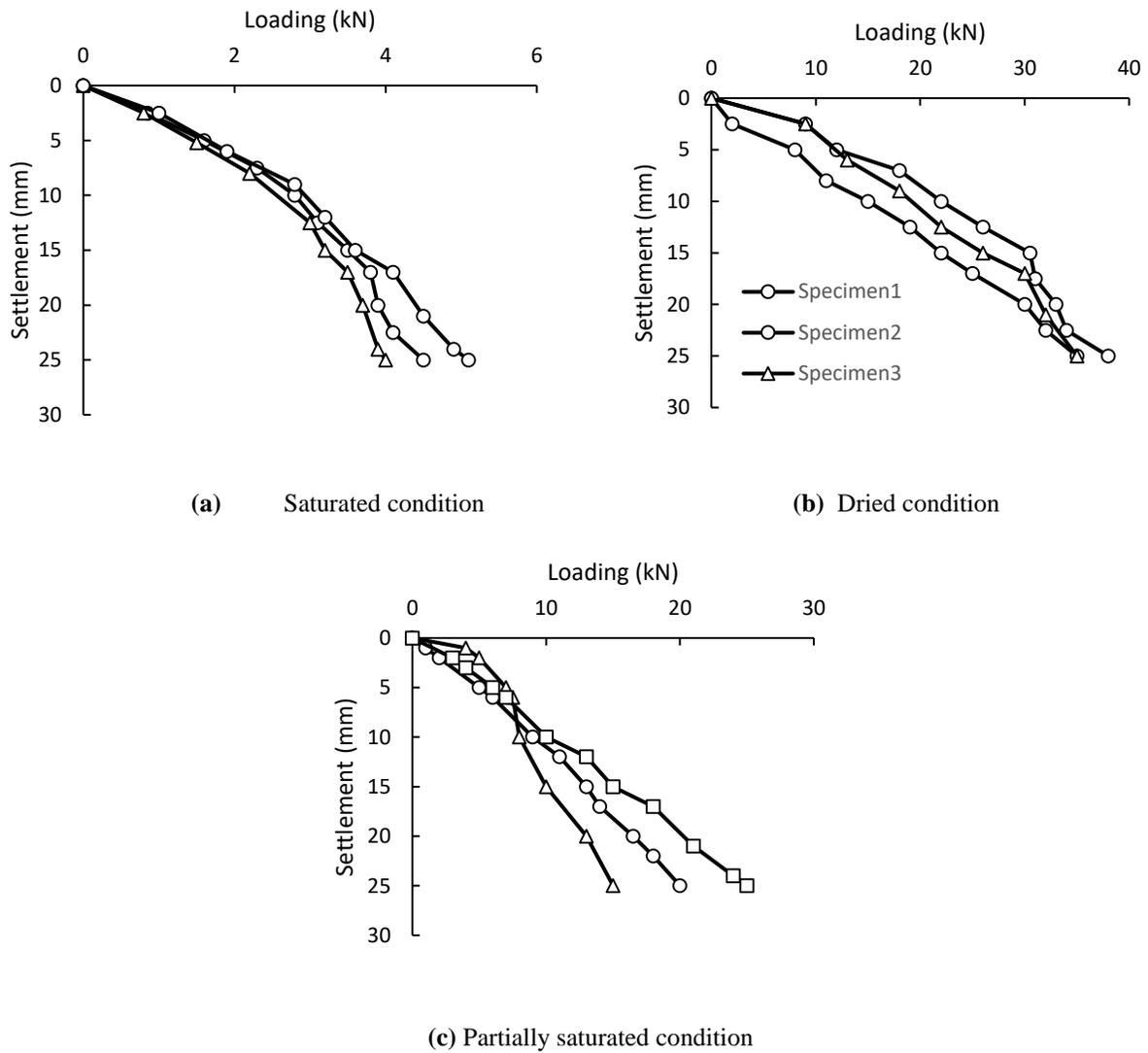
**Fig. 11.** Load-settlement behavior of CLM column (column alone loaded) specimens
