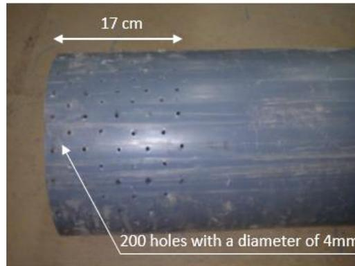
Fig. 2. Perforated polyethylene pipe
