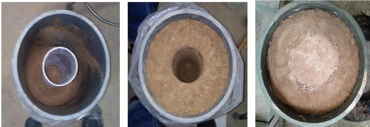
(a) Compacted soil layer and pipe on the second layer
