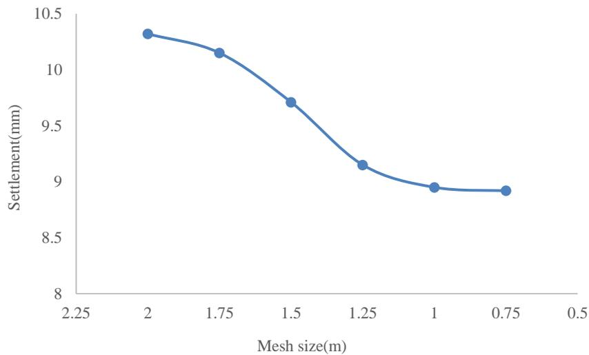
**Fig. 2.** Mesh convergence analysis for the FE model
