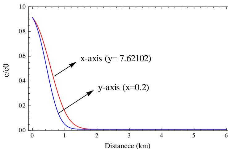
**Fig.13.** Calculated contaminant concentration obtained with Eq. (37) for line sources along the distance  $x$  and  $y$  -axes respectively at the end of 5 years
