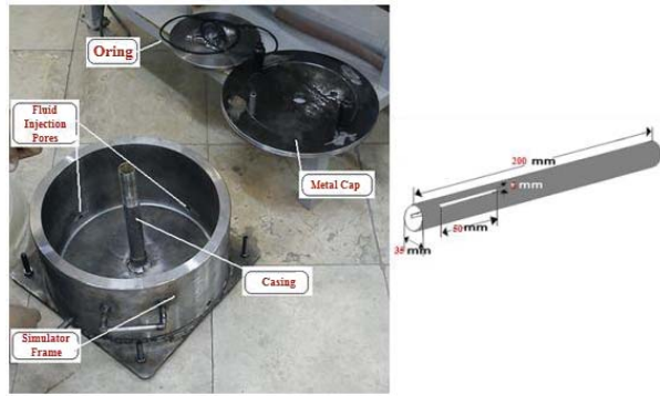
Figure 4. Chamber of reservoir simulator with the cover and interior components [9]
