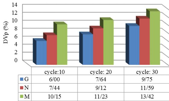
Figure 9. Ultrasound wave velocity index (DVp) against cycle (C) in stations (G, N, M, and their average)
