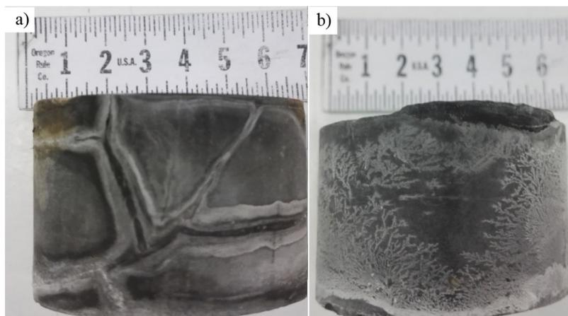
Figure 4. Effect of weak planes on the penetration depth of salt: a) a jointed slate and b) an intact slate
