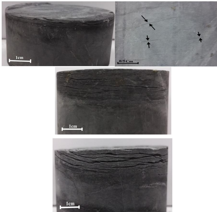
Figure 5. Visible changes on foliation due to salt crystallization cycles (10, 20, and 30).
