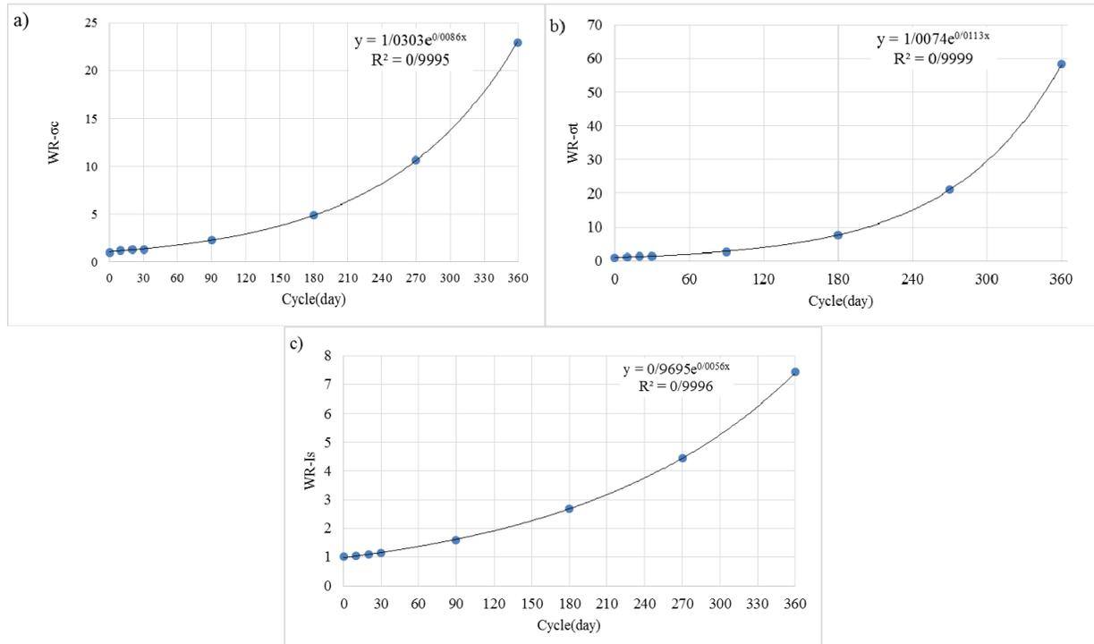
Figure 10. Relationships between *WR* and cycle (day): a) uniaxial compressive strength ( $\sigma_c$ ), b) Brazilian test ( $\sigma_t$ ), and c) Point load index (*Is*)
