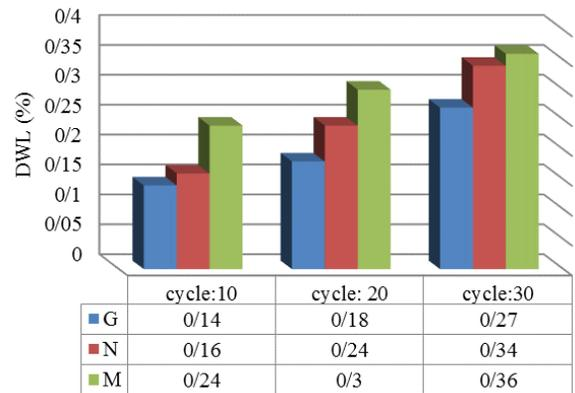
Figure 8. Dry weight loss (DWL) against cycle (C) in stations (G, N, M, and their average)
