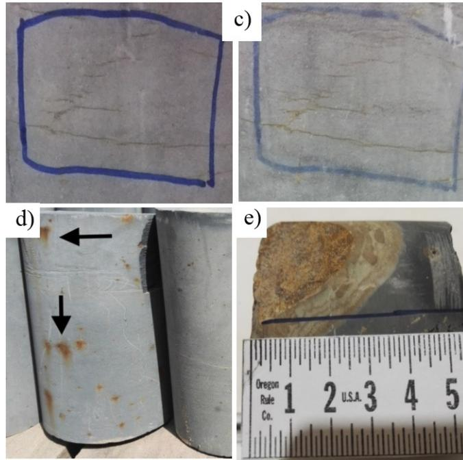
Figure 7. Observable changes due to weathering: a) cycles 10, b) cycles 20, c) cycles 30, d) short-term natural weathering, and e) long-term natural weathering condition
