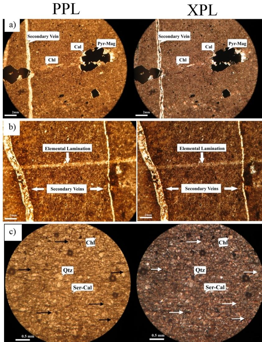
Figure 3. Photomicrographs of rock samples: a) Station N (parallel to the foliation), b) Station M (parallel to the foliation), and c) Station G (perpendicular to the foliation) (*Cal*: Calcite, *Qtz*: Quartz, *Chl*: Chlorite, *Pyr-Mag*: pyrite-Magnetite, and *Ser*: serresite).
