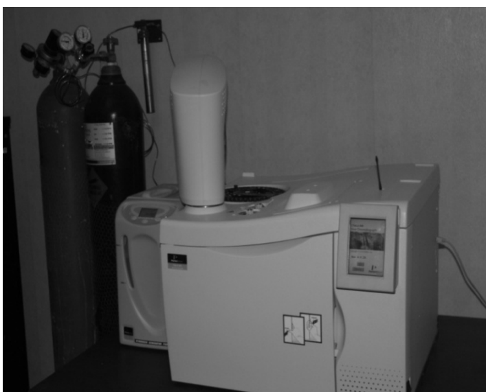
Fig. 2. The Gas Chromatograph used for oil and produced biodiesel analysis
