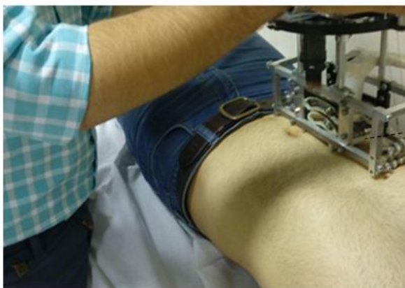
Figure 11 Experimental evaluation of maintaining contact between probe and patient's body
