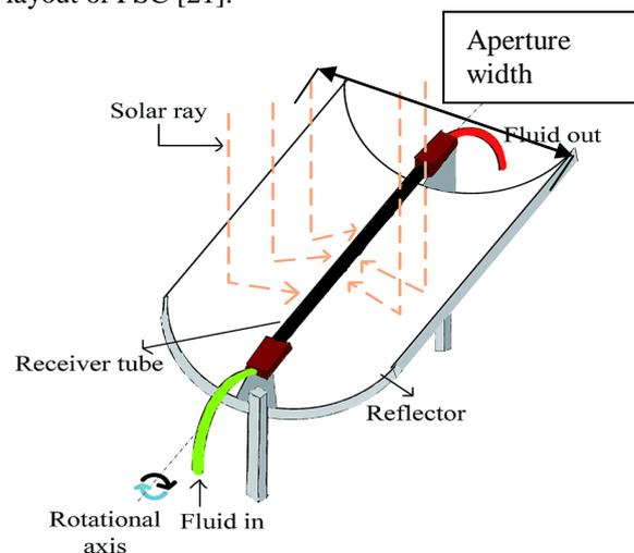
**Figure 1** – Parabolic solar collector with absorber/receiver pipe
