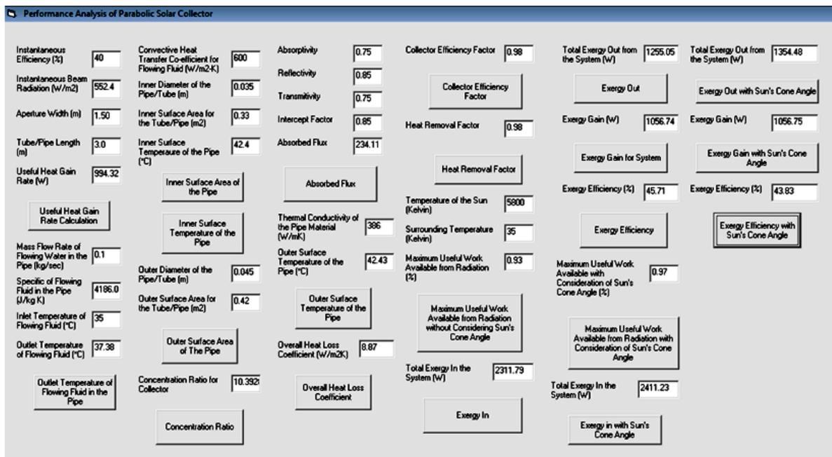
Figure 2 – PAPSC Software for performance analyses of PSC at various conditions with/without Sun's cone angle
