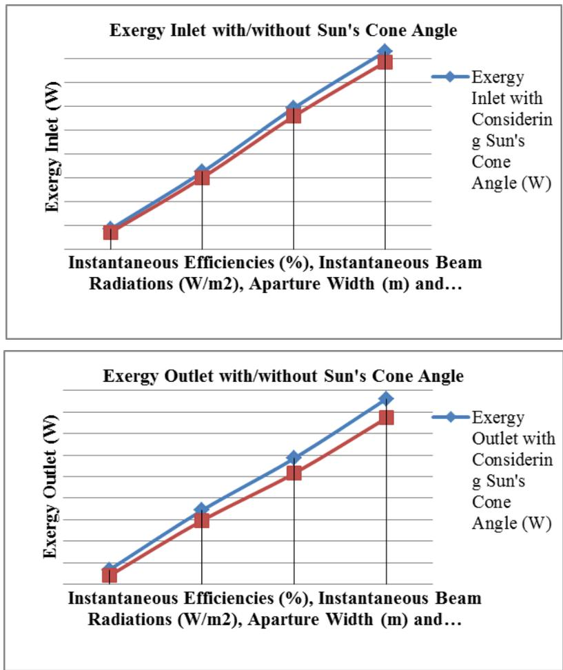
**Figure 6** – (a) Exergy inlet and (b) exergy outlet with/without considering sun’s cone angle at different  $\eta_i$ , IR, B and  $l_e$  conditions
