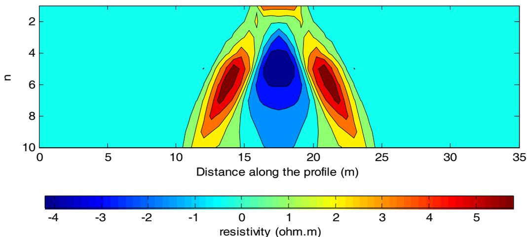
Figure 4. Difference of pseudo-sections for the block with its depth to top equal to 0.5 m.
