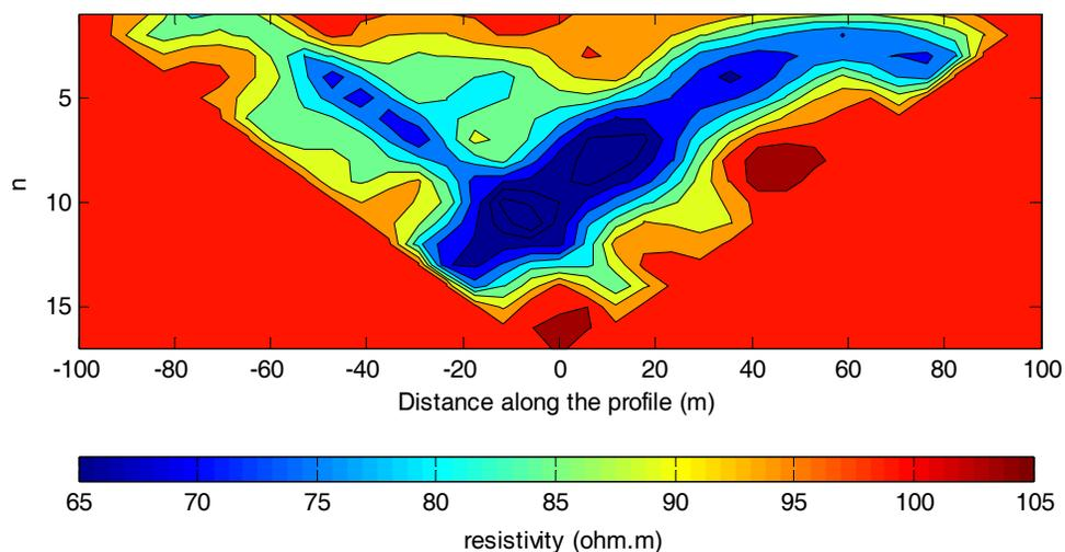
**Figure 7.** Pseudo-section obtained by RES2DMOD software. Comparing this standard result with IE one is expressive of the productivity of IE method.
