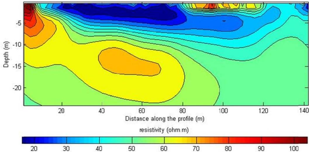
**Figure 12.** Inversed model by applying the IE code on landfill data with the RMS error of 4.5%.
