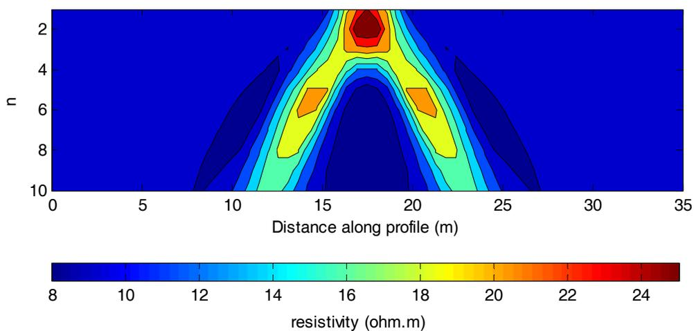
**Figure 2.** Pseudo-section derived from IE method when depth to top of the block is 0.5 m. Data sampling interval and dipole separation both were 1 m. Symmetry can be observed from this pseudo-section.
