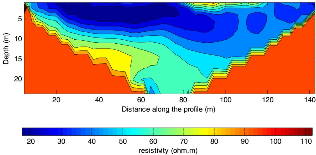
**Figure 11.** Recovered model by RES2DINV software with the RMS error of 2.3 %. Reconstructed model is in a good agreement with the true model.
