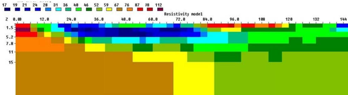
Figure 9. True model of the landfill that can be found between default models of RES2DMOD software.
