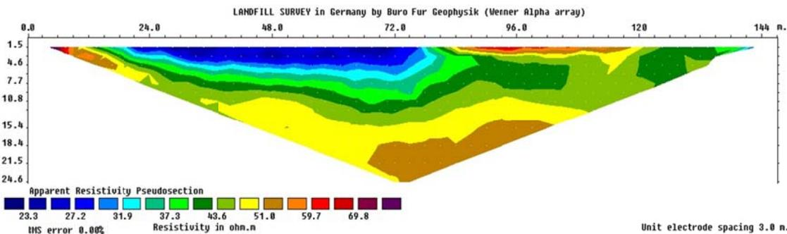
Figure 10. Pseudo-section of the landfill model. Two dipole separations were used: 3 m with n from 1 to 8 and 6 m with n from 5 to 8. This representation of the RES2DMOD software is just for dipole separation of 3 m.
