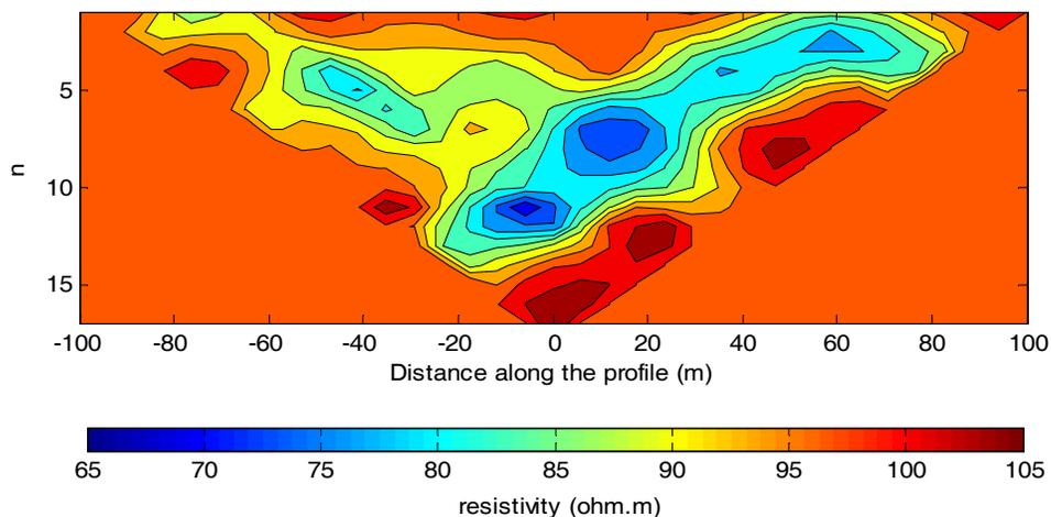
**Figure 6.** Pseudo-section calculated by IE method. It is difficult to find a single block response and they incline to be mixed with nearby anomalies.
