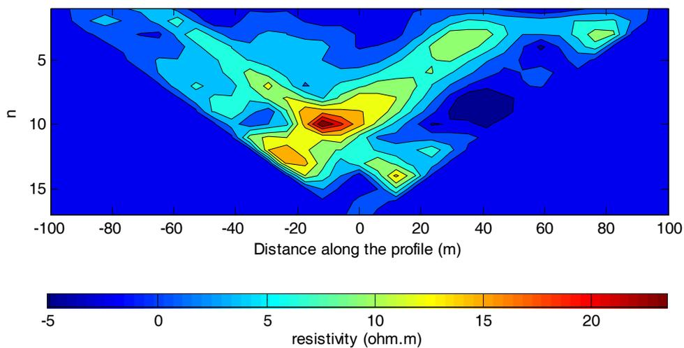
**Figure 8.** Difference of two pseudo-sections. For  $n=10$  and approximately in the middle of the array, the largest error is occurred.
