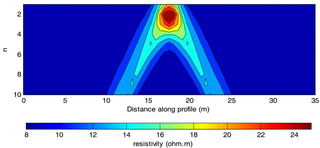
**Figure 3.** Pseudo-section derived from RES2DMOD software when depth to top of the block is 0.5 m. Data sampling interval and dipole separation both were 1 m. As the result of IE, it also shows a symmetry.
