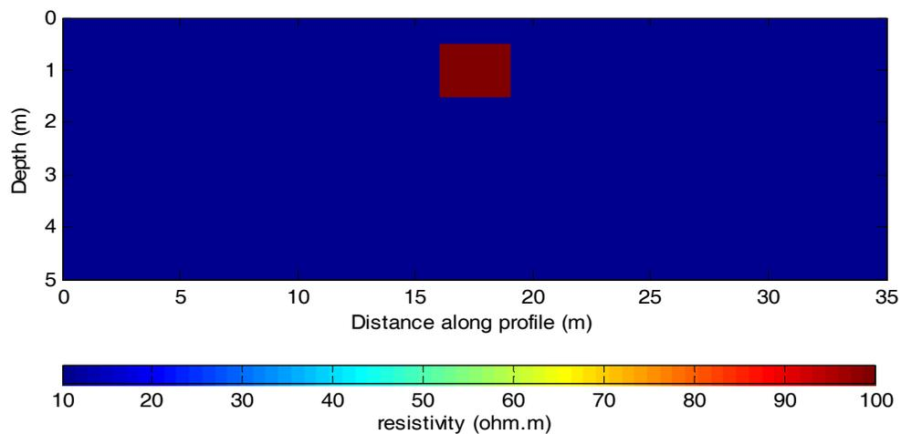
**Figure 1.** Model of a resistive block surrounded by a homogeneous medium that is a simple model for DC resistivity method.
