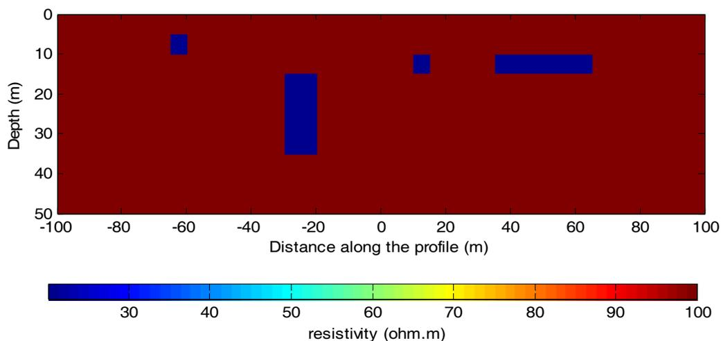
Figure 5. Four conductive bodies immersed in a resistive host medium that can be considered as a complex resistivity model.
