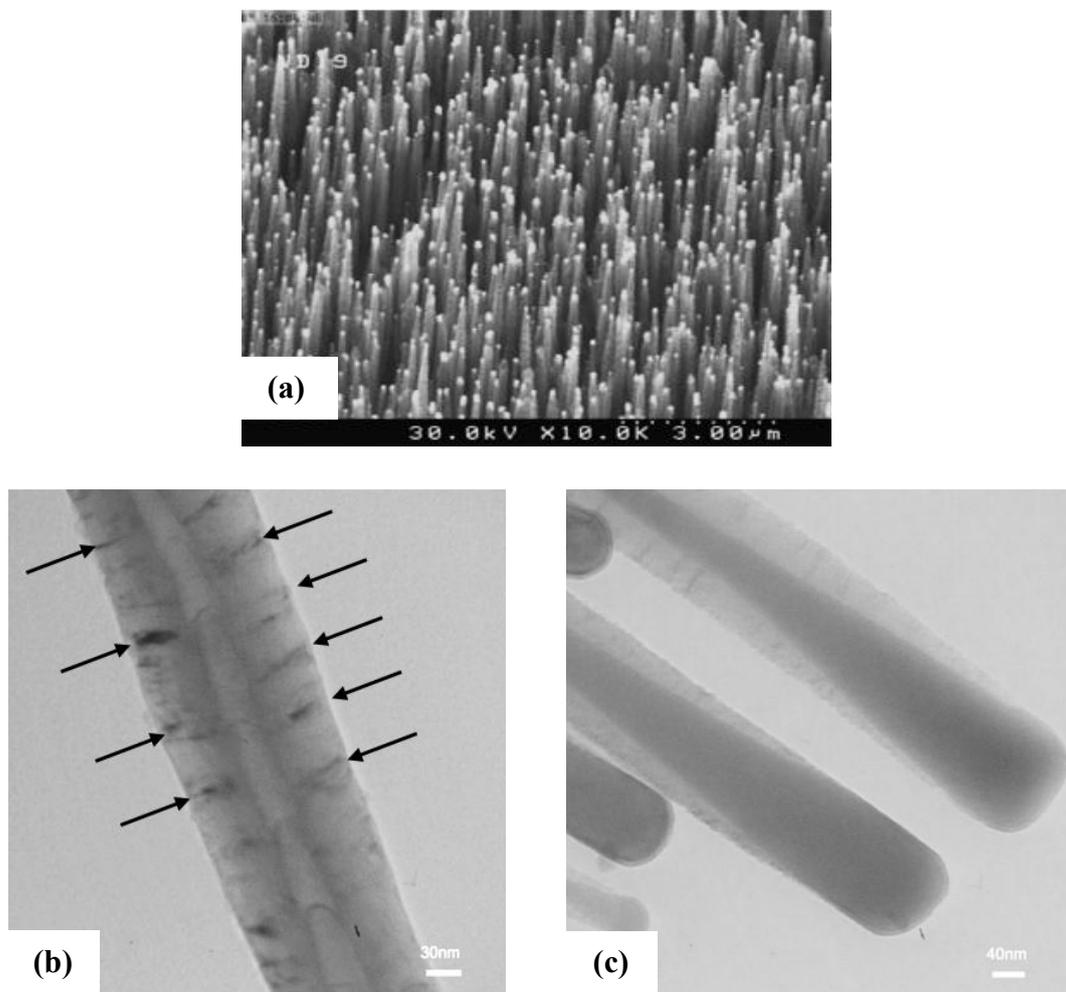
Fig. 2- (a)SEM and (b) TEM image of Nitrogen doped CNTs. (c) TEM image of bare CNTs without N-doping.
