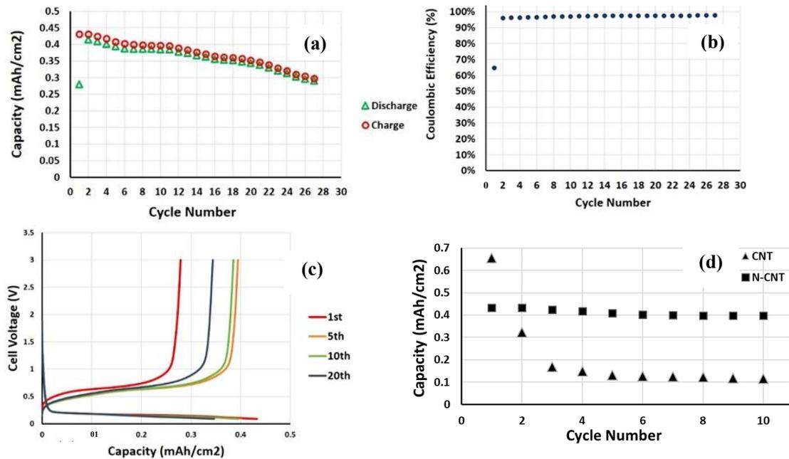
Fig. 3- The results of charge/discharge test for the Lithium ion battery. (a) Specific capacity for 28 cycles with current of 100  $\mu$ A, in the potential range of 50 m to 3 V. (b) Coulombic efficiency of the cell. (c) Cell voltage profile. (d) Specific capacity in the first 10 cycles for both bare CNT and Nitrogen doped CNT based Lithium ion batteries. N-doped sample presents 4 times higher capacity at final cycles.
