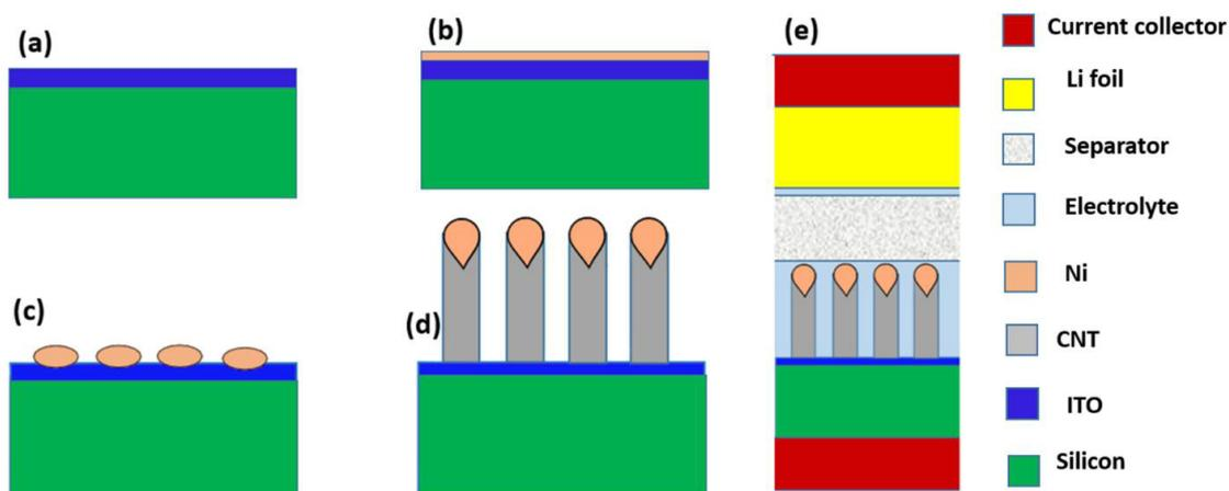
Fig. 1- Schematic presentation of CNT growth and Lithium ion battery components. (a) ITO coated Silicon substrate. (b) Nickel deposition on the substrate. (c) Forming Nickel islands, (d) Growth of CNTs and (e) Fabrication of Lithium ion battery.
