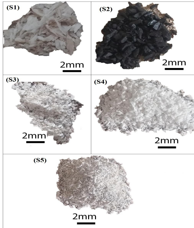
Fig. 1- The changes of dog bone colors during the heat treatment and MW irradiation for S1: Raw bone; S2: Raw bone after heating at 600 °C for 150 min; S3: Sample after 10 min MW irradiation and then heating at 600 °C for 150 min; S4: Sample after 10 min MW irradiation and then heating at 900 °C for 150 min; S5: Sample after 30 min MW irradiation.
