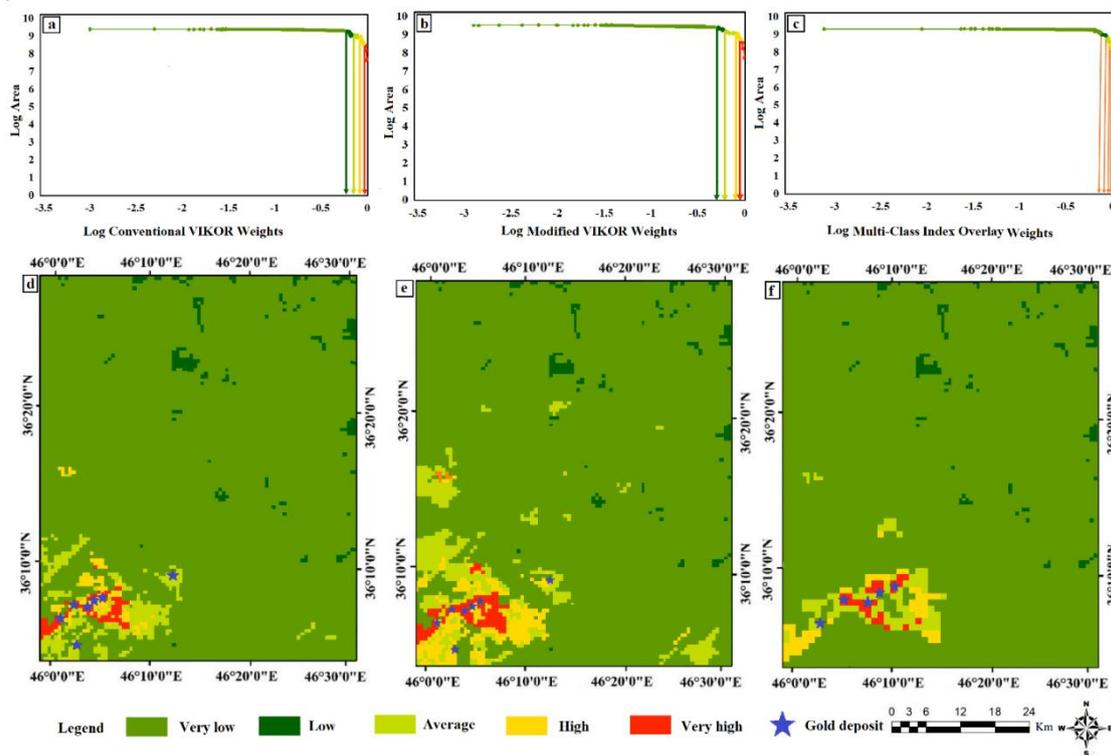
Figure 10. Gold prospectivity/potential maps prepared by applying the VIKOR and multi-class index overlay approaches. The C-A multi-fractal curves for reclassifying the outputs are depicted in the left column, and the final potential maps are illustrated in the right column, while (a), (b) are for conventional VIKOR, (c), (d) for modified VIKOR, and (e) and (f) for multi-class index overlay.
