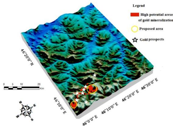
Figure 11. The digital elevation map of the Saez prospecting zone depicted in 3D, on which the most favorable zones for gold mineralization were superimposed.
