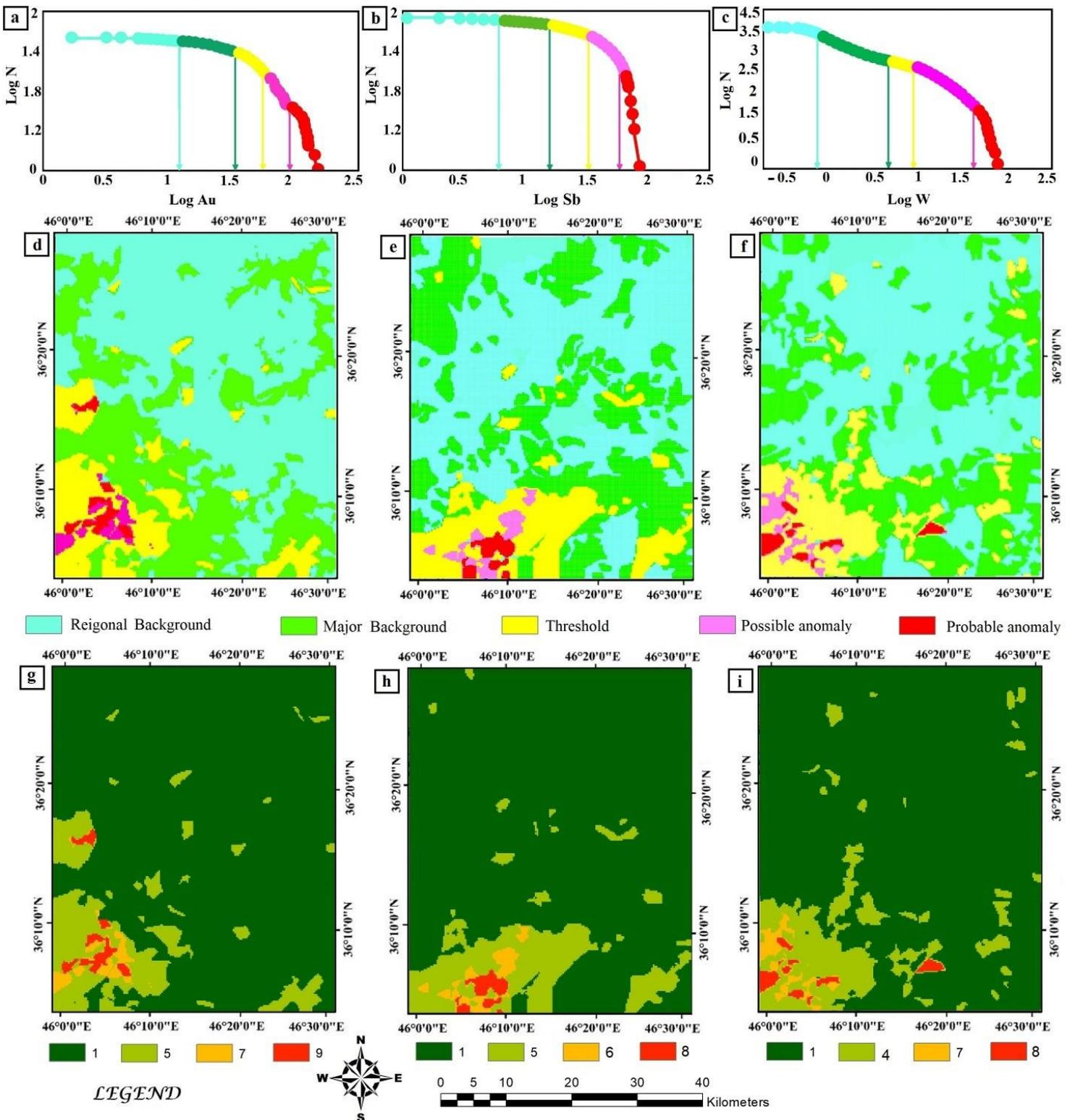
Figure 8. The log-log plots of C-N multi-fractal curves of stream sediment geochemical data for Au, Sb, and W (top row), the reclassified concentration maps based on the derived thresholds (middle row), and the geochemical indicator maps for three elements (bottom row).
