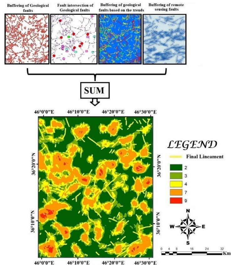
Figure 4. Final tectonic indicator layer showing the importance of geological lineaments in gold exploration. This map was generated by implementing a SUM operator to four sub-groups of structural features.
