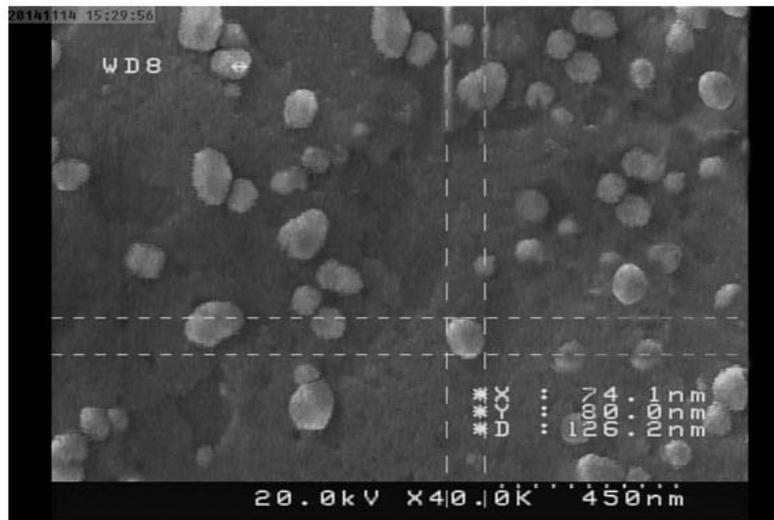
Fig. 2. SEM images of insulin loaded nanoparticles.
