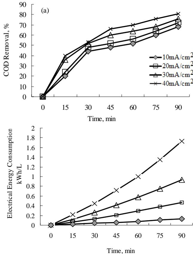
Fig. 2. Effect of the current density on COD removal efficiency (a), and on electrical energy consumption (b).
