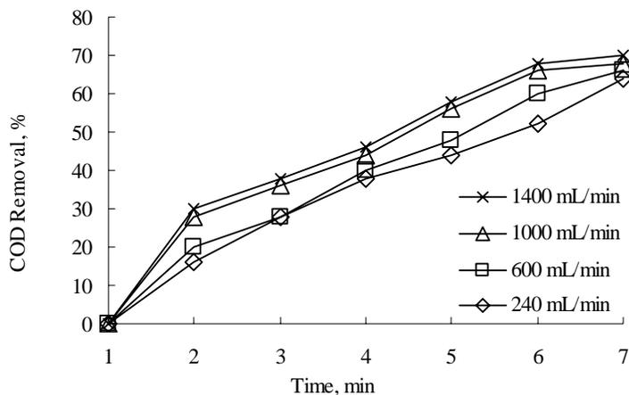
Fig. 4. Effect of the flow rate on COD concentrations: Current density: 40 mA/cm<sup>2</sup>, pH:7.1, 0.1M Na<sub>2</sub>SO<sub>4</sub>.
