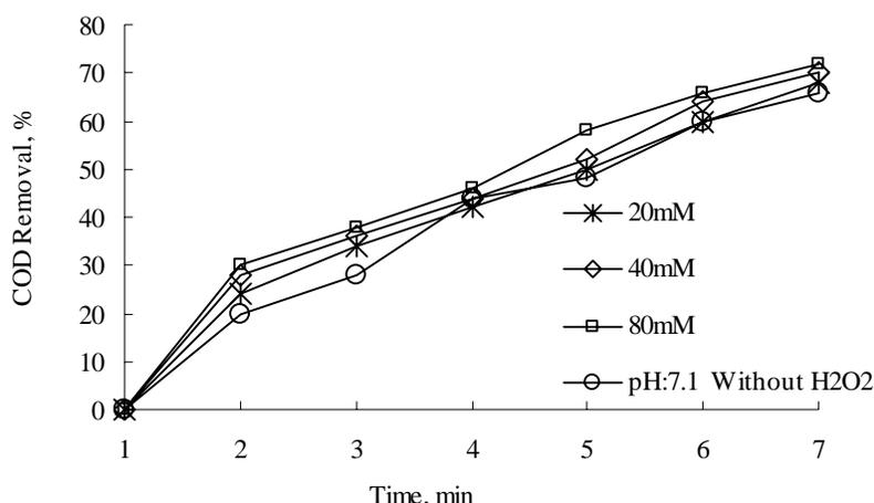
Fig. 6. The effect of  $H_2O_2$  on COD removal efficiency. pH:3,  $v_{\text{circulate}}$ : 600mL/min, 0.1M  $Na_2SO_4$ , Current Density: 40 mA/cm<sup>2</sup>
