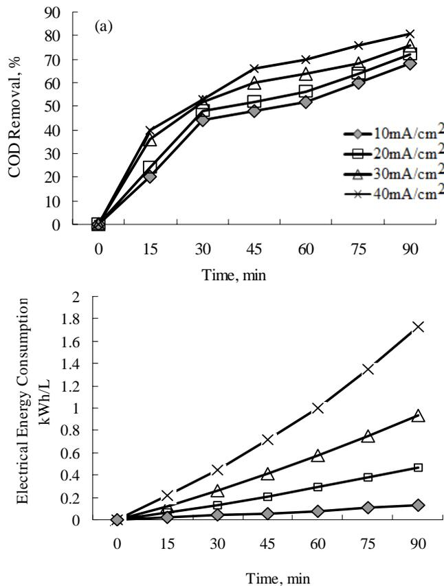
**Fig. 2. Effect of the current density on COD removal efficiency (a), and on electrical energy consumption (b).**
