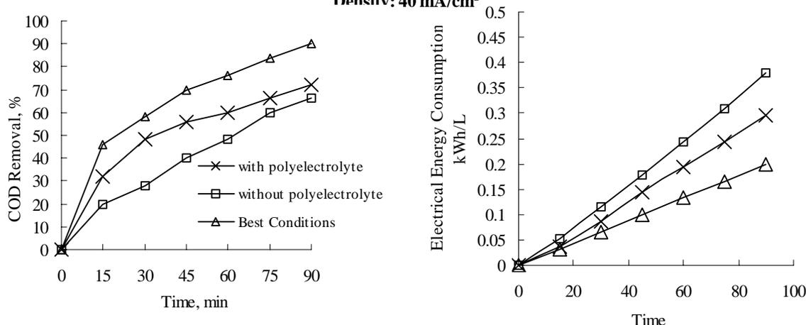
Fig. 7. Effect of the polyelectrolyte and operation under best conditions (a) on COD concentrations and (b) on electrical energy consumption.
