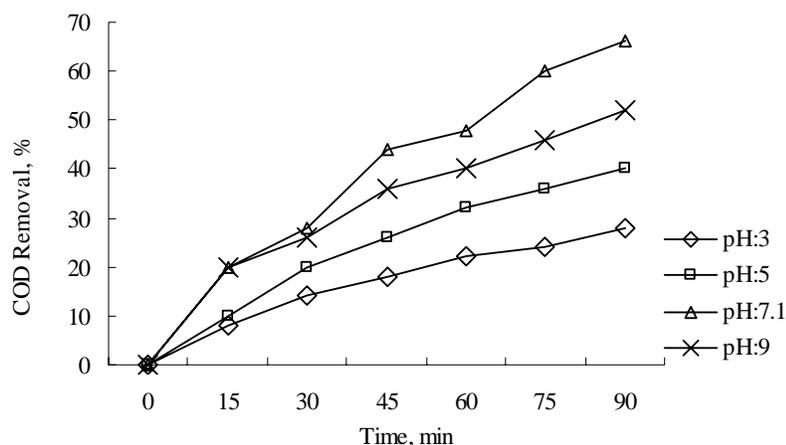
**Fig. 5. Effect of the pH on COD removal efficiency.  $v_{\text{circulate}}$ : 600mL/min, 0.1M Na<sub>2</sub>SO<sub>4</sub>, Current Density: 40 mA/cm<sup>2</sup>**
