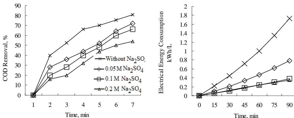
**Fig. 3.** The effect of supporting electrolyte (a) on COD concentrations and (b) on electrical energy consumption.  $v_{\text{circulate}}: 600 \text{ mL/min}$ , pH 7.1, Current Density:  $40 \text{ mA/cm}^2$
