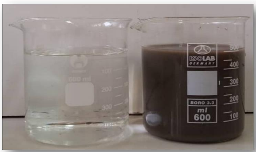
Fig. 7. Appearance of wastewater and reactor's output
