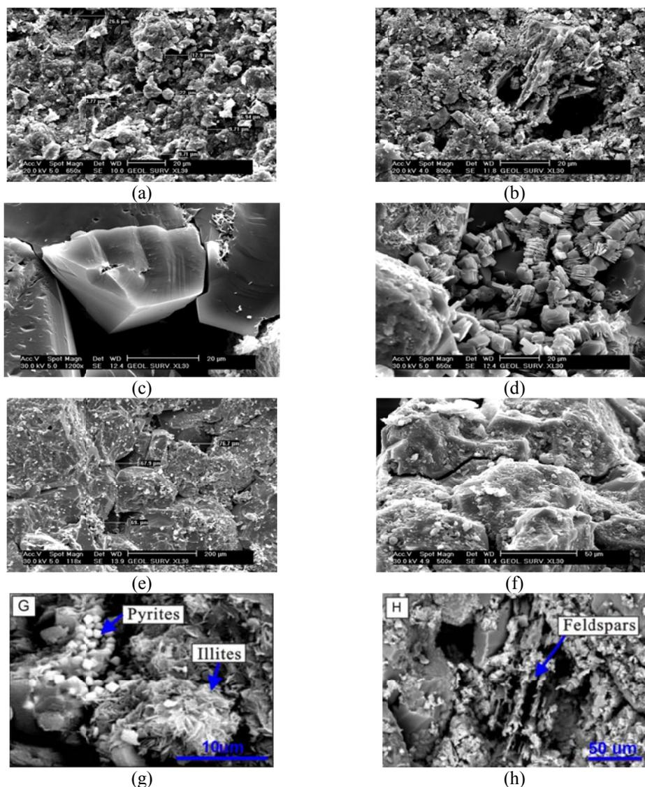
**Figure 2.** a) Anisotropic flattened pore spaces, b) Anisotropic pores filled with clay flakes, c) Completely mature quartz grains and pore spaces, d) Authigenic kaolinite booklets with some pores, e) Isotropic and anisotropic pore spaces, f) Anisotropic zigzag tortoise, g) Crystallized illites with pyrite crystals, h) Secondary intragranular dissolved pores between grains with silica overgrowths.
