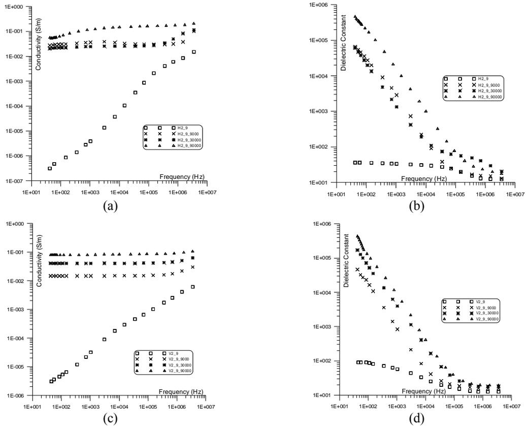
Figure 11. The conductivity and dielectric constant of sample (9) measured in horizontal (bedding plane direction (a, b)) and vertical (perpendicular to the bedding plane (c, d)) directions.
