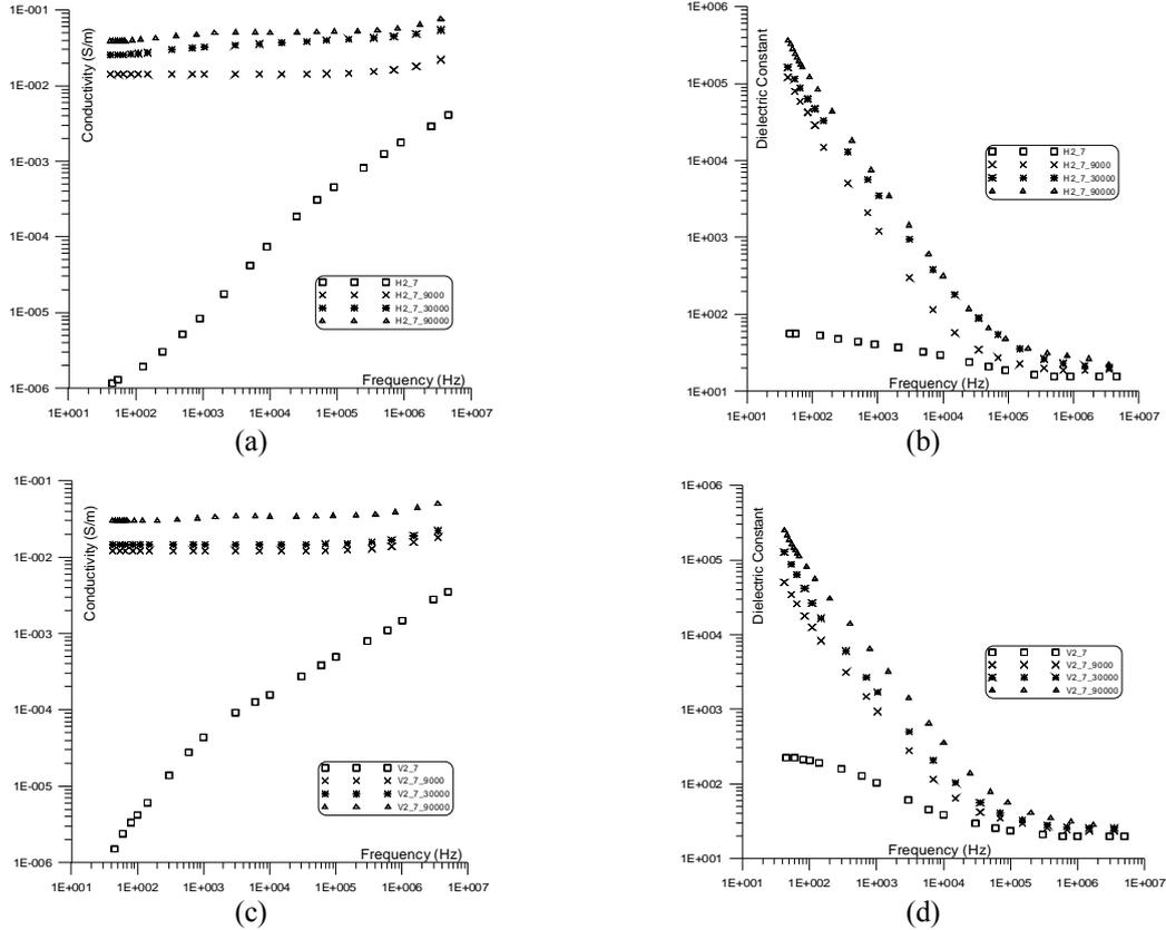
Figure 10. The conductivity and dielectric constant of sample (7) measured in horizontal (bedding plane direction (a, b)) and vertical (perpendicular to the bedding plane (c, d)) directions.
