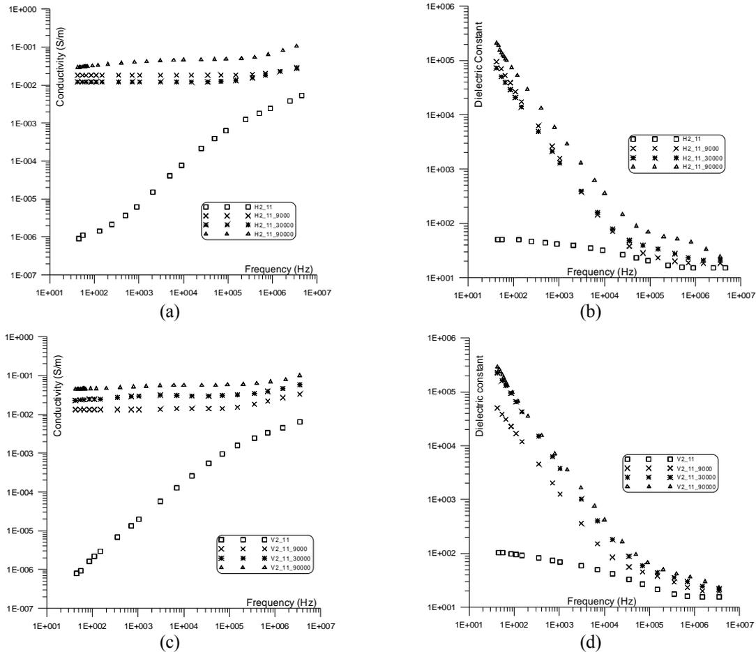
**Figure 12.** The conductivity and dielectric constant of sample (11) measured in horizontal (bedding plane direction (a, b)) and vertical (perpendicular to the bedding plane (c, d)) directions.
