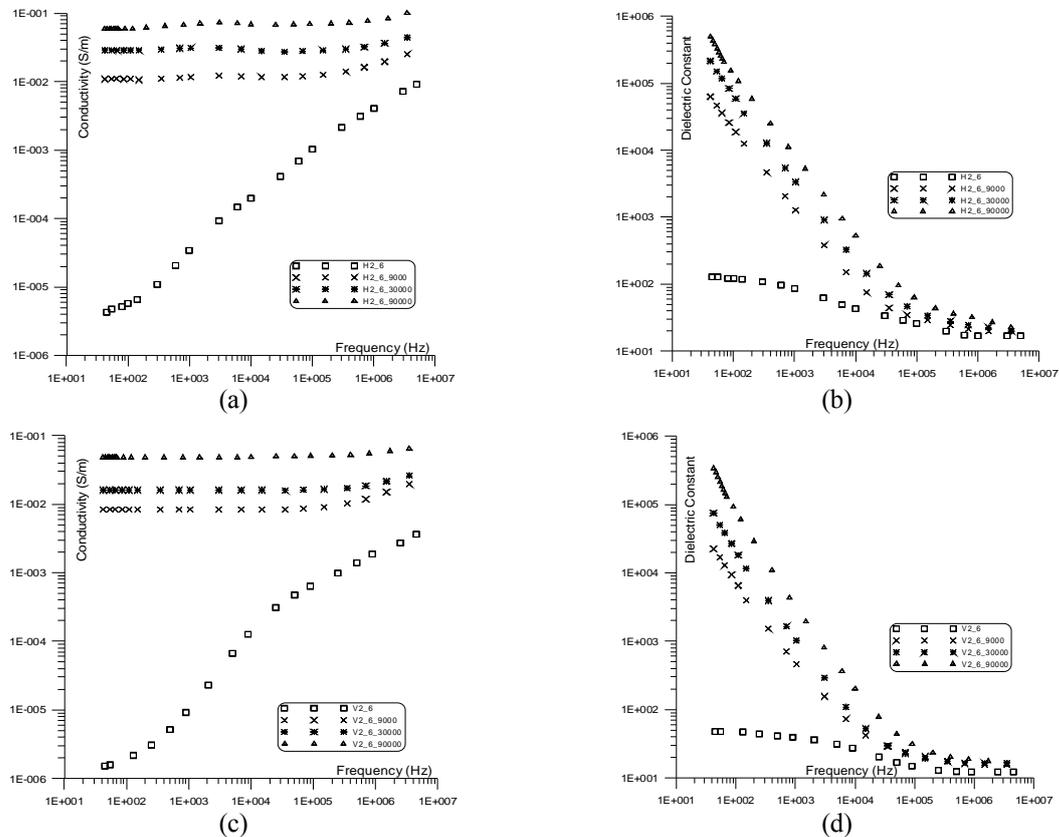
Figure 9. The conductivity and dielectric constant of sample (6) measured in horizontal (bedding plane direction (a, b)) and vertical (perpendicular to the bedding plane (c, d)) directions.
