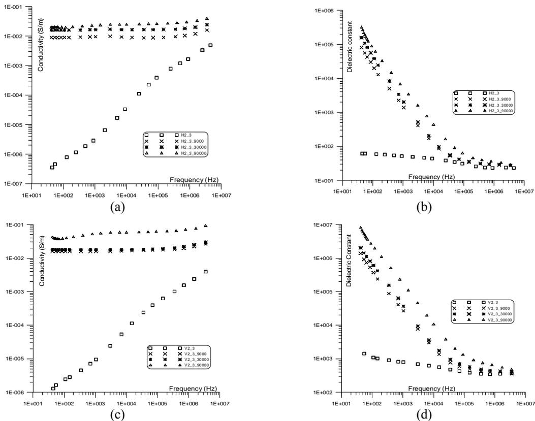
Figure 6. The conductivity and dielectric constant of sample (3) measured in horizontal (bedding plane direction (a, b)) and vertical (perpendicular to the bedding plane (c, d)) directions.
