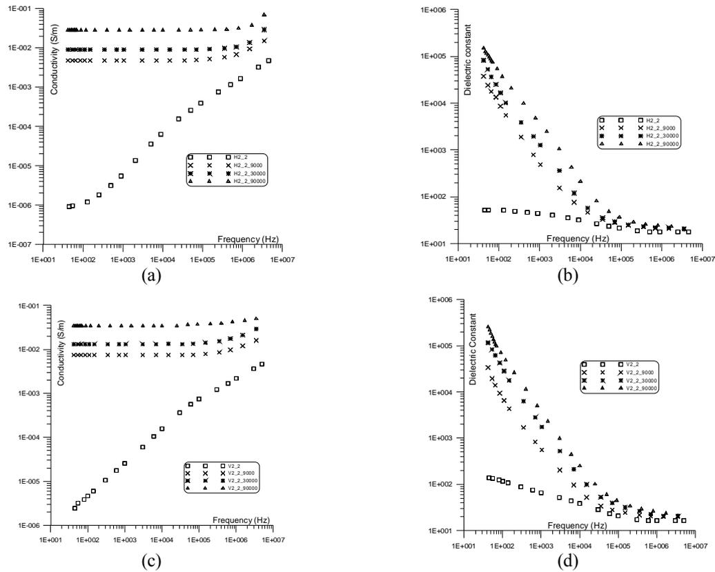
Figure 5. The conductivity and dielectric constant of sample (2) measured in horizontal (bedding plane direction (a, b)) and vertical (perpendicular to the bedding plane (c, d)) directions.
