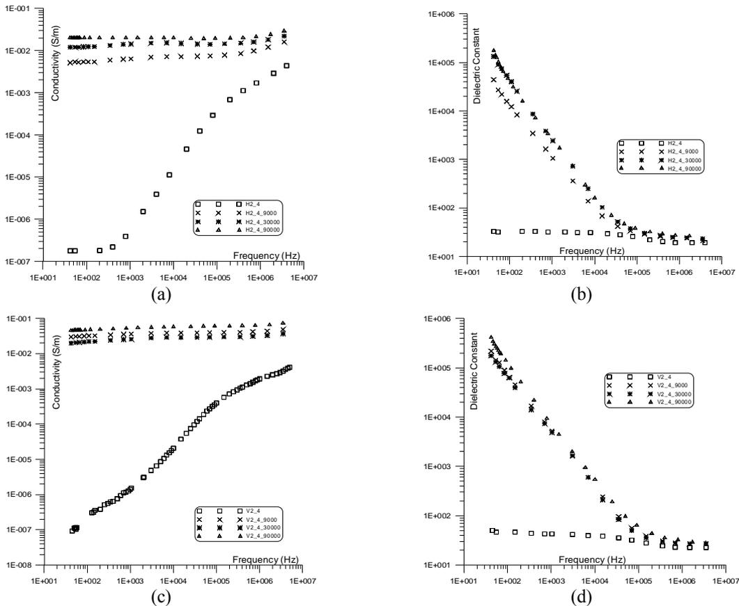
Figure 7. The conductivity and dielectric constant of sample (4) measured in horizontal (bedding plane direction (a, b)) and vertical (perpendicular to the bedding plane (c, d)) directions.
