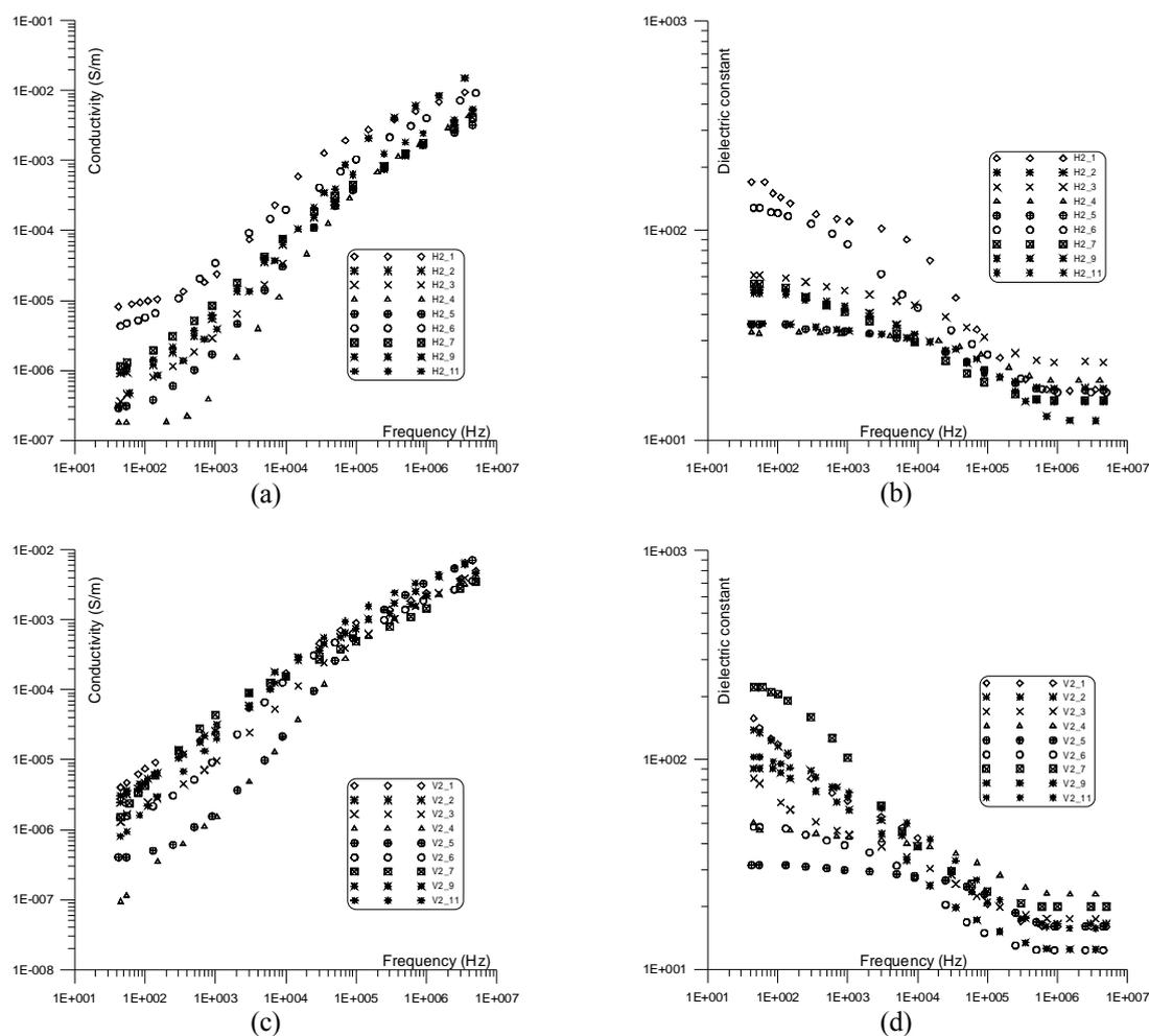
**Figure 3.** The conductivity and dielectric constant of samples measured (dry) in horizontal (bedding plane direction (a, b)) and vertical (perpendicular to the bedding plane (c, d)) directions.
