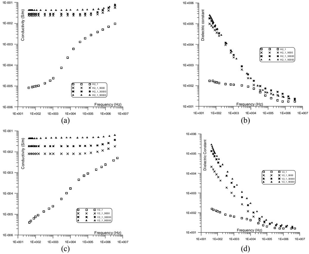
Figure 4. The conductivity and dielectric constant of sample (1) measured in horizontal (bedding plane direction (a, b)) and vertical (perpendicular to the bedding plane (c, d)) directions.
