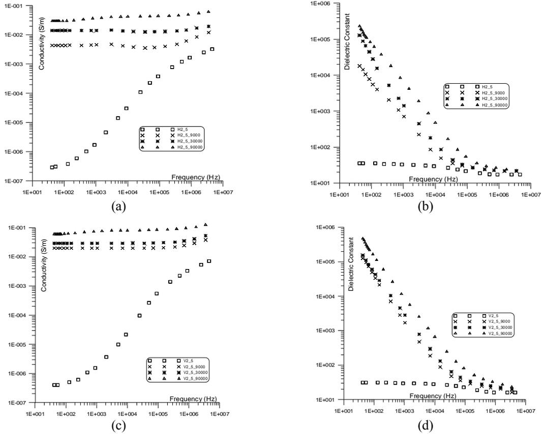
Figure 8. The conductivity and dielectric constant of sample (5) measured in horizontal (bedding plane direction (a, b)) and vertical (perpendicular to the bedding plane (c, d)) directions.
