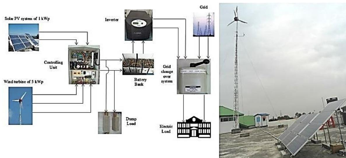
**Fig. 1. Schematic and actual solar/wind hybrid system setup at rooftop of CEEE, NIT Hamirpur.**
