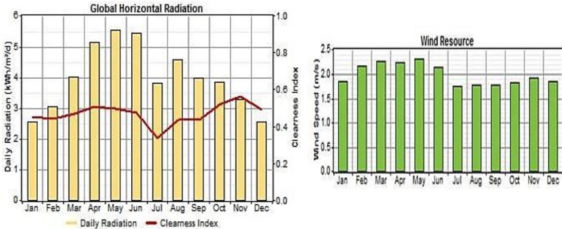
Fig. 4. Monthly average global solar radiation and wind speed at CEEE, Hamirpur (H.P)
