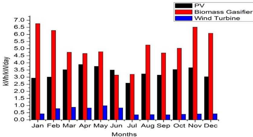
Fig. 8. Normalized daily energy production for PV, BM and Wind.
