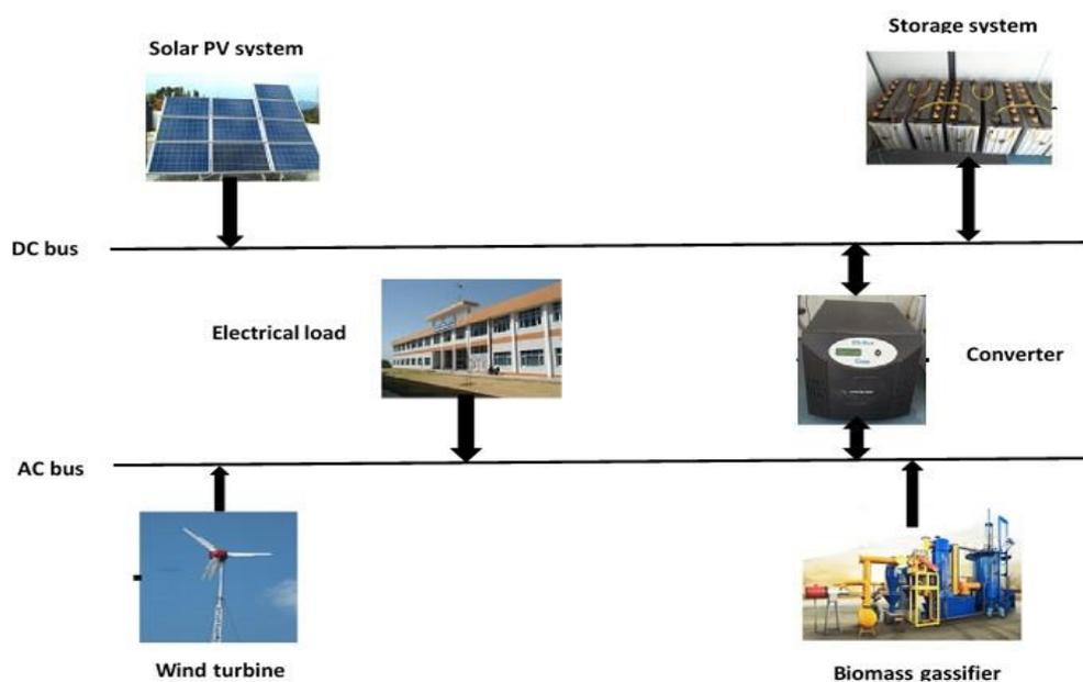
**Fig. 2. The schematic diagram of proposed hybrid energy system.**
