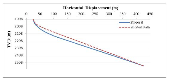
Figure 8: Comparison between proposed & shortest well path
