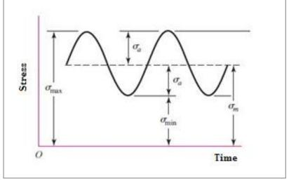
Figure 4: Stress-Time relation, fluctuating stress[8]
