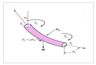
Figure 2: Drill string in curved section
