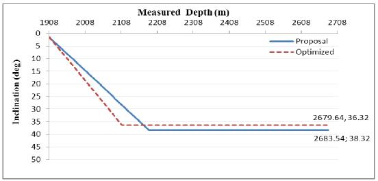
Figure 10: Maximum well angle measured depth, the slope represents the dogleg severity.
