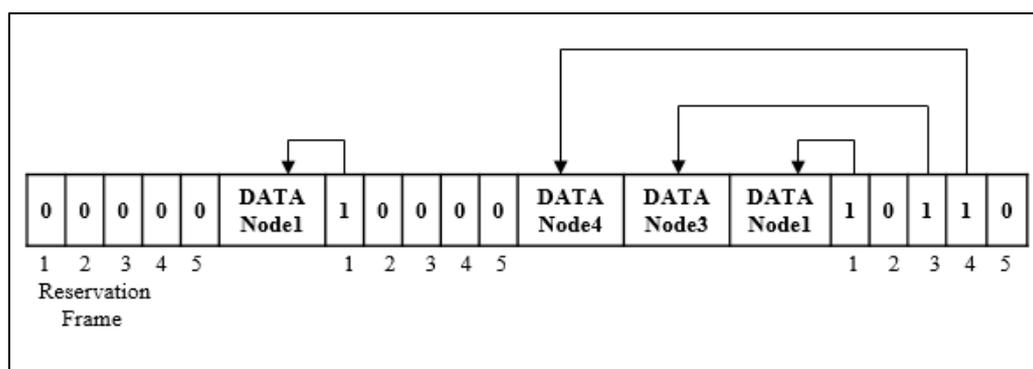
Figure 2. Situation of five nodes and five slot reservation frames
