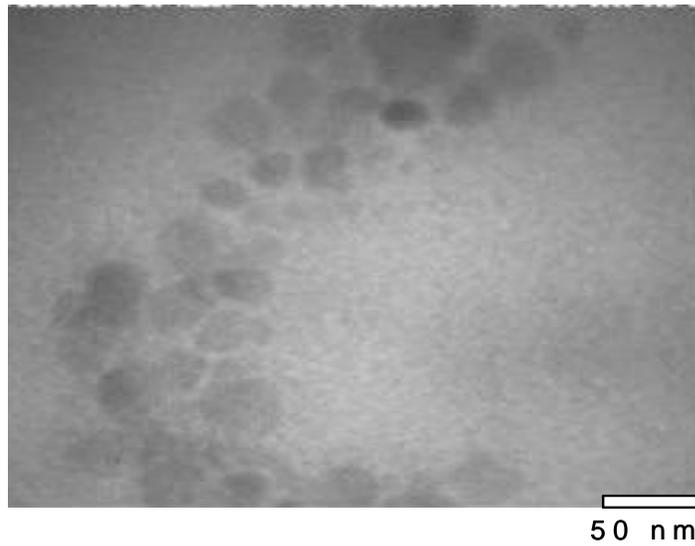
Fig.3. The TEM image taken from iron magnetic nanoparticles synthesized in this study
