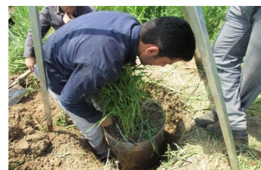
Figure 1. The way of taking undisturbed soil core with inner container of the lysimeter at two land uses of alfalfa and wheat
