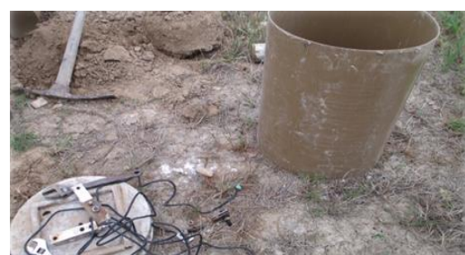
Figure 2. The outer container of lysimeter and metal foundation to install the loadcell
