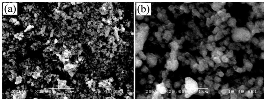
Fig. 4- FESEM images of ((a) 5 KX; (b) 20 KX) of the CrN/Cu composite powders.
