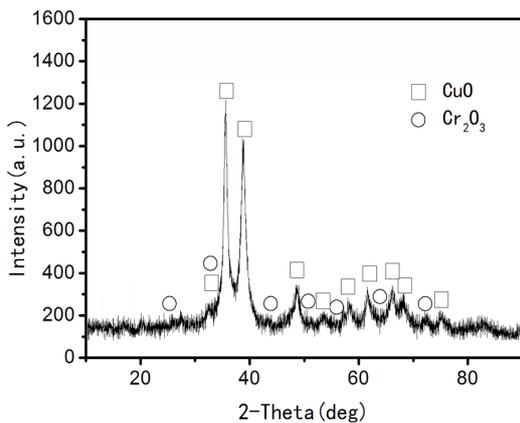
Fig. 1- XRD pattern of the precursor prepared from  $\text{Cr}(\text{NO}_3)_3$  with a concentration of 0.005 mol/L in the solution.
