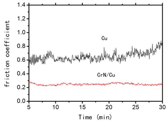
Fig. 5- The friction coefficient of the pure copper and CrN/Cu composite specimens.
