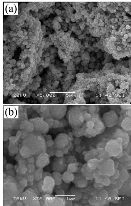
Fig. 2- FESEM images ((a) 5 KX; (b) 20 KX) of the precursor prepared from  $\text{Cr}(\text{NO}_3)_3$  with a concentration of 0.005 mol/L in the solution.
