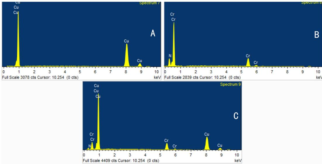
Fig. 9- EDS results of the corresponding areas in Fig. 8b.
