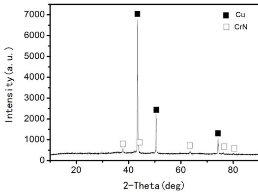
Fig. 3- XRD pattern of the calcined CrN/Cu composite powders.
