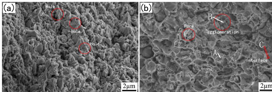
Fig. 8- FESEM photographs of the fractured surfaces of the sintered pure Cu (a) and CrN/Cu composite (b) samples.
