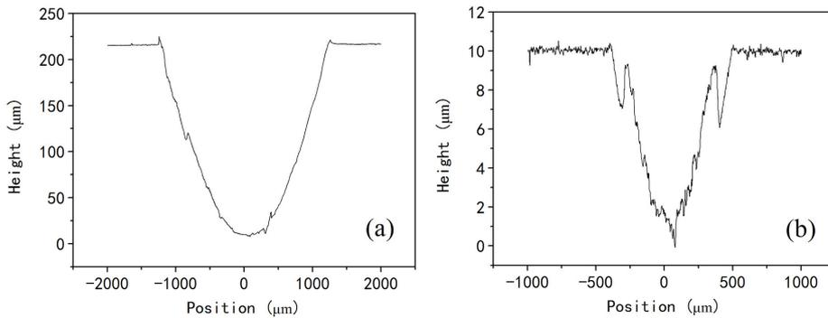
Fig. 7- Cross-sectional profiles of the wear tracks of the sintered pure Cu (a) and CrN/Cu composite (b) samples.
