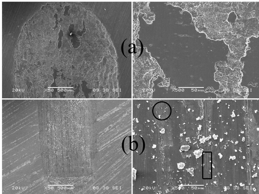
Fig. 6- SEM micrographs of worn surface of the sintered pure copper (a) and CrN/Cu composite (b) specimens.
