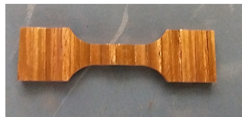
Fig. 5- Prepared Sample for Tensile Test.
