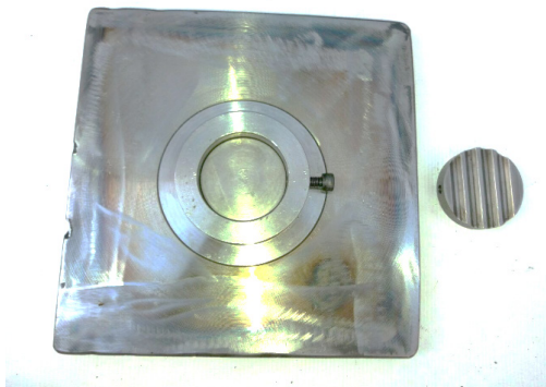
Fig. 2- Fixture and bottom part of flat and grooved molds.
