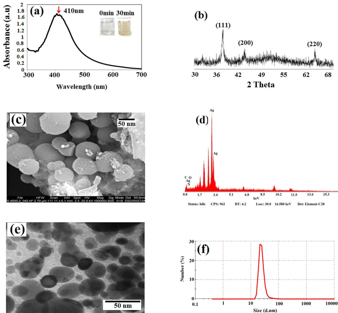
Fig. 1- (a) UV-Visible, (b) XRD, (c) ESEM, (d) EDS spectrum (e) TEM image and (f) DLS of the synthesis of AgNPs using MO.
