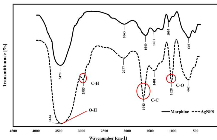
Fig. 2- FTIR spectrum for MO and AgNPs.
