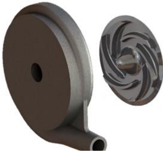
Figure 6. 3D model of the impeller and volute.
