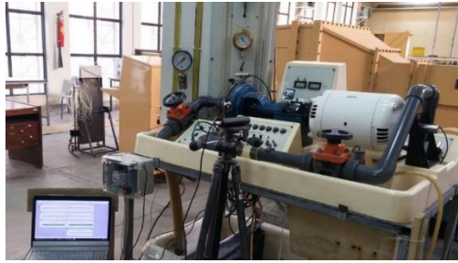
Figure 1. Centrifugal pump test-rig and the data acquisition system.
