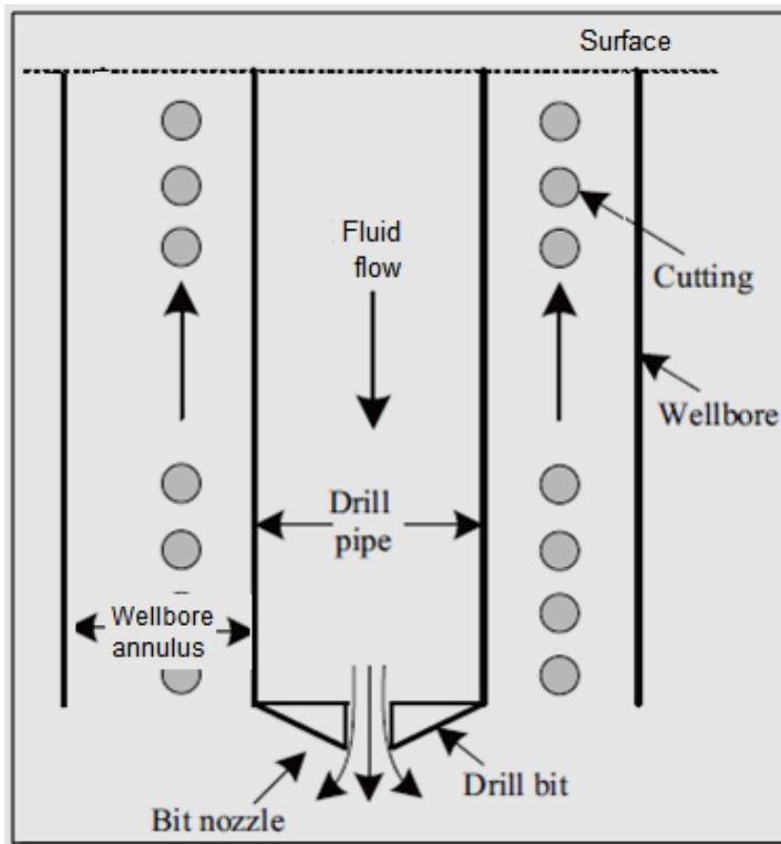
**Fig. 1.** Schematic of cuttings transport in a vertical-section
