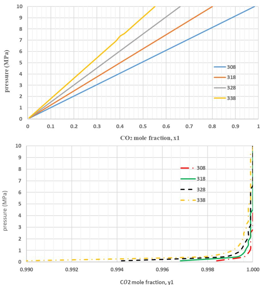
Fig. 4. Comparison of VLE of DMSO–CO<sub>2</sub> system calculated according to PR at 308, 318, 328, and 338 K
