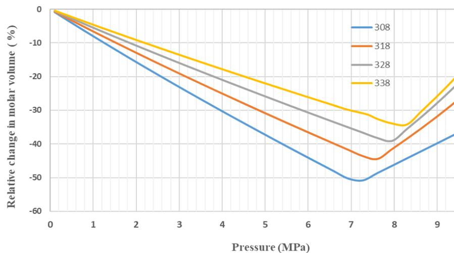
**Fig. 3.** Relative expansion of the liquid phase as a function of pressure, calculated according to PR for the systems DMSO–CO<sub>2</sub> at different temperature (308, 318, 328, and 338 K)
