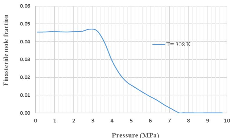
**Fig. 5.** The calculated solubility of FNS in the liquid phase expanded by supercritical CO<sub>2</sub> for the ternary system of CO<sub>2</sub>-DMSO-finasteride at 308 K
