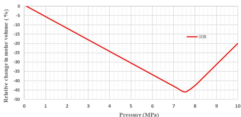
**Fig. 6.** Relative expansion of the liquid phase as a function of pressure, calculated according to PR for the systems DMSO-CO<sub>2</sub>-FNS at 308 K
