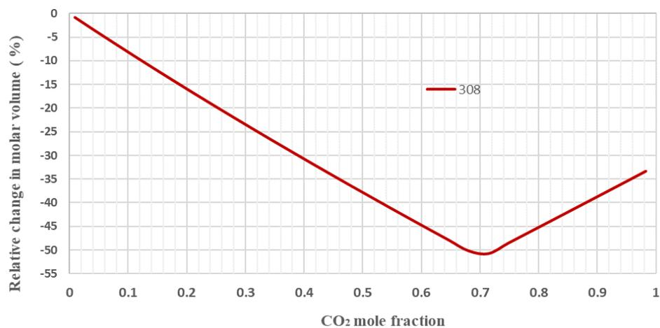
**Fig. 2.** Relative expansion of the liquid phase as a function of CO<sub>2</sub> mole fraction in the liquid phase, calculated according to PR for the systems DMSO–CO<sub>2</sub> at 308 K
