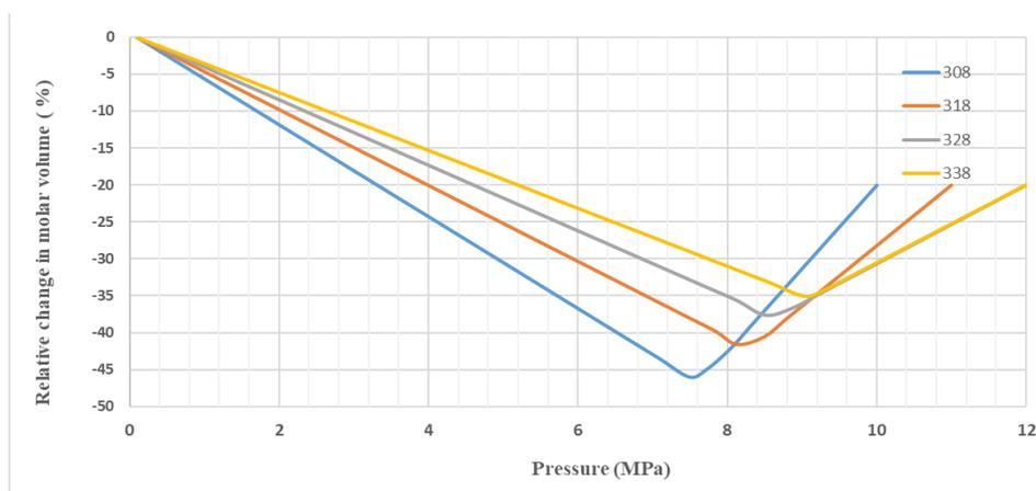
**Fig. 7.** Relative expansion of the liquid phase as a function of pressure, calculated according to PR for the systems CO<sub>2</sub>–DMSO–FNS at different temperature (308, 318, 328, and 338 K)
