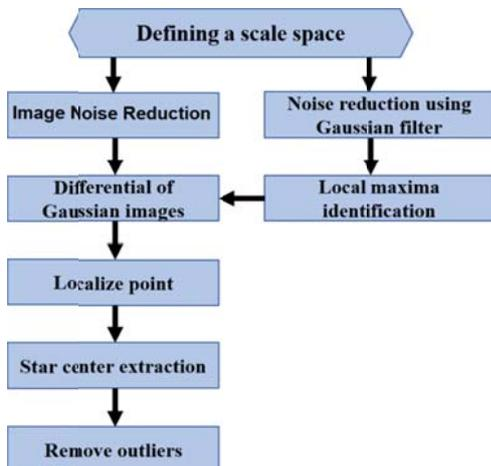
**Figure 2.** Star recognition process using SIFT algorithm.
