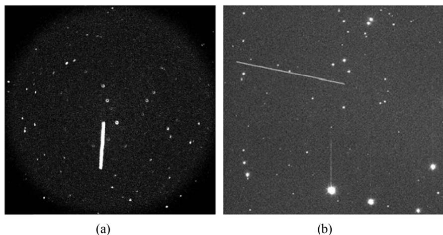
**Figure 4.** sample images used in this study using Ixon Ultra 888 CCD with different Exposure time a) 0.5 sec and b) 1 sec.
