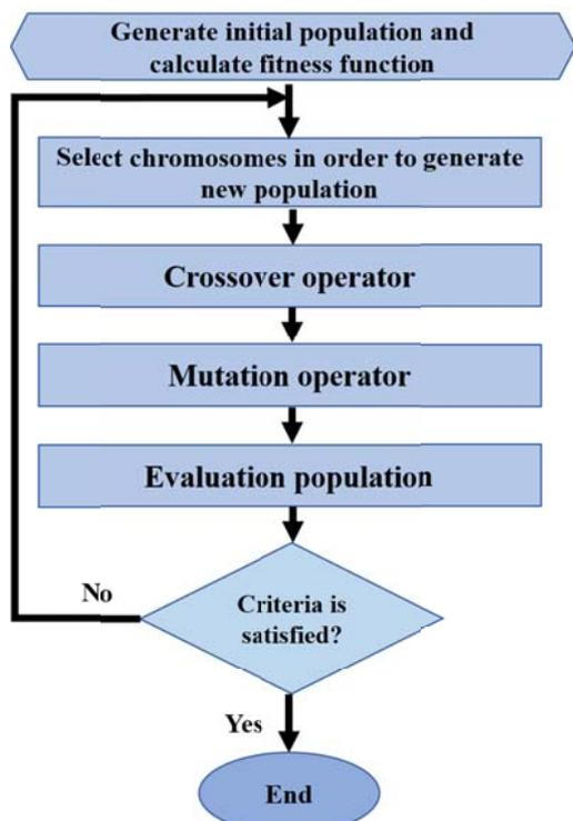
**Figure 3.** General overview of Genetic algorithm procedure during satellite's streak detection.
