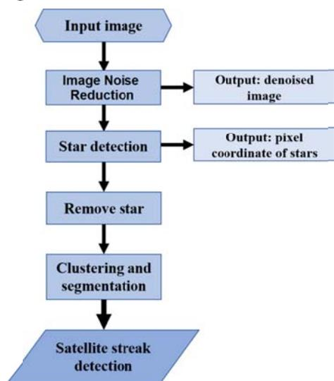
**Figure 1.** General procedure for satellite's streak detection.
