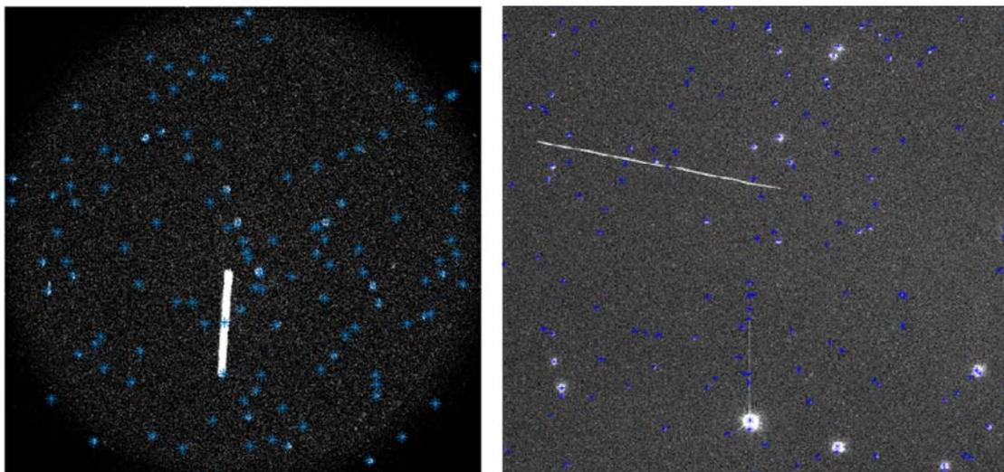
Figure 7. Display of star's center pixel coordinate using SIFT algorithm.
