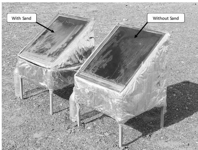
Figure 2. Image of the solar stills used in the experiment
