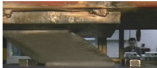
Fiber reinforced elastomeric isolator Sp. No. 3 G. Dehghani & A. Aghakouchak T.M.U., IRAN
