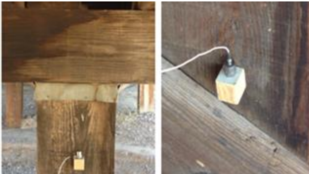
Fig. 6. Accelerometers mounted on piles using wooden blocks
