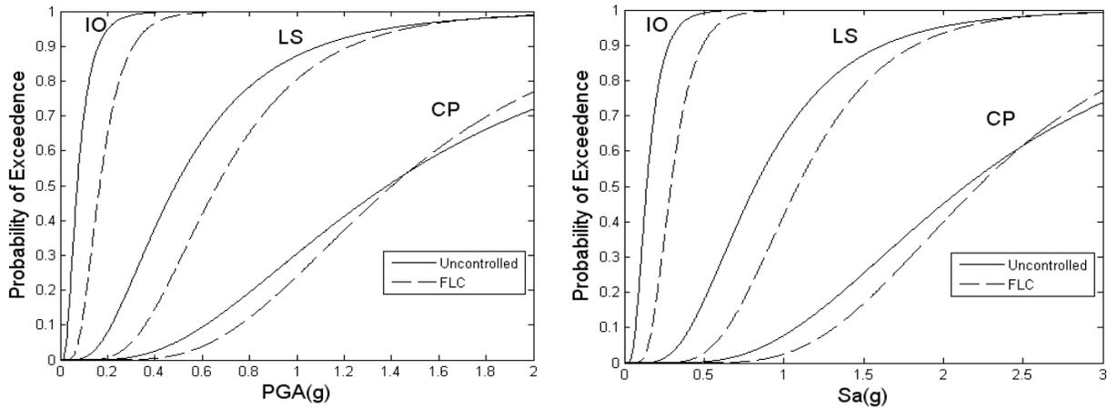
Fig. 4. Comparing fragility curves for uncontrolled and fuzzy logic controller
