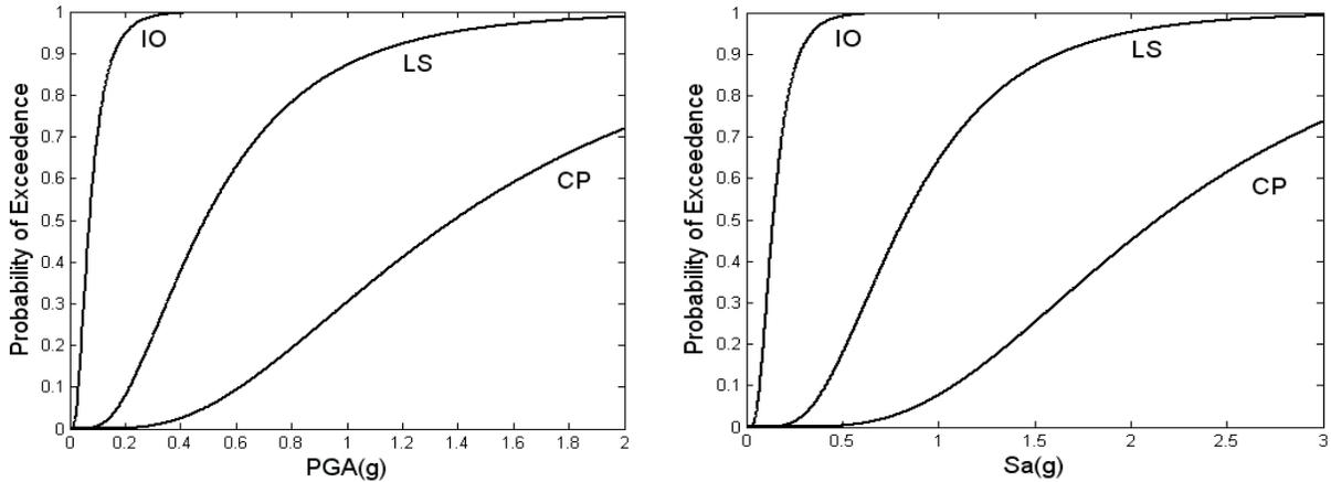
**Fig. 2.** Fragility curves for uncontrolled structure
