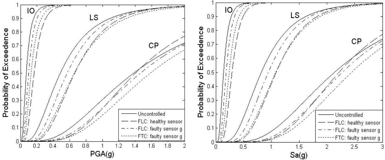
Fig. 10. Fragility curves for different controllers (fault can occur in sensor of ground)
