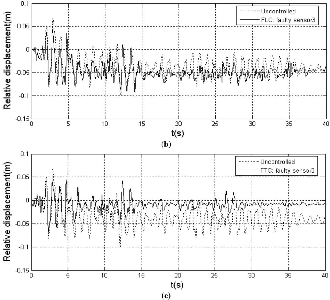
**Fig. 11.** Relative displacement response of story 3 under El Centro earthquake: a) comparing uncontrolled and FLC when are sensors are healthy; b) comparing uncontrolled and FLC when sensor 3 is faulty; c) comparing uncontrolled and FTC when sensor 3 is faulty
