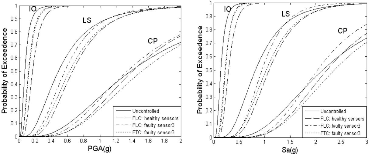
Fig. 9. Fragility curves for different controllers (fault can occur in sensor of story 3)
