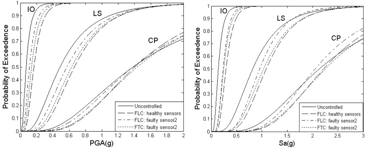
Fig. 8. Fragility curves for different controllers (fault can occur in sensor of story 2)
