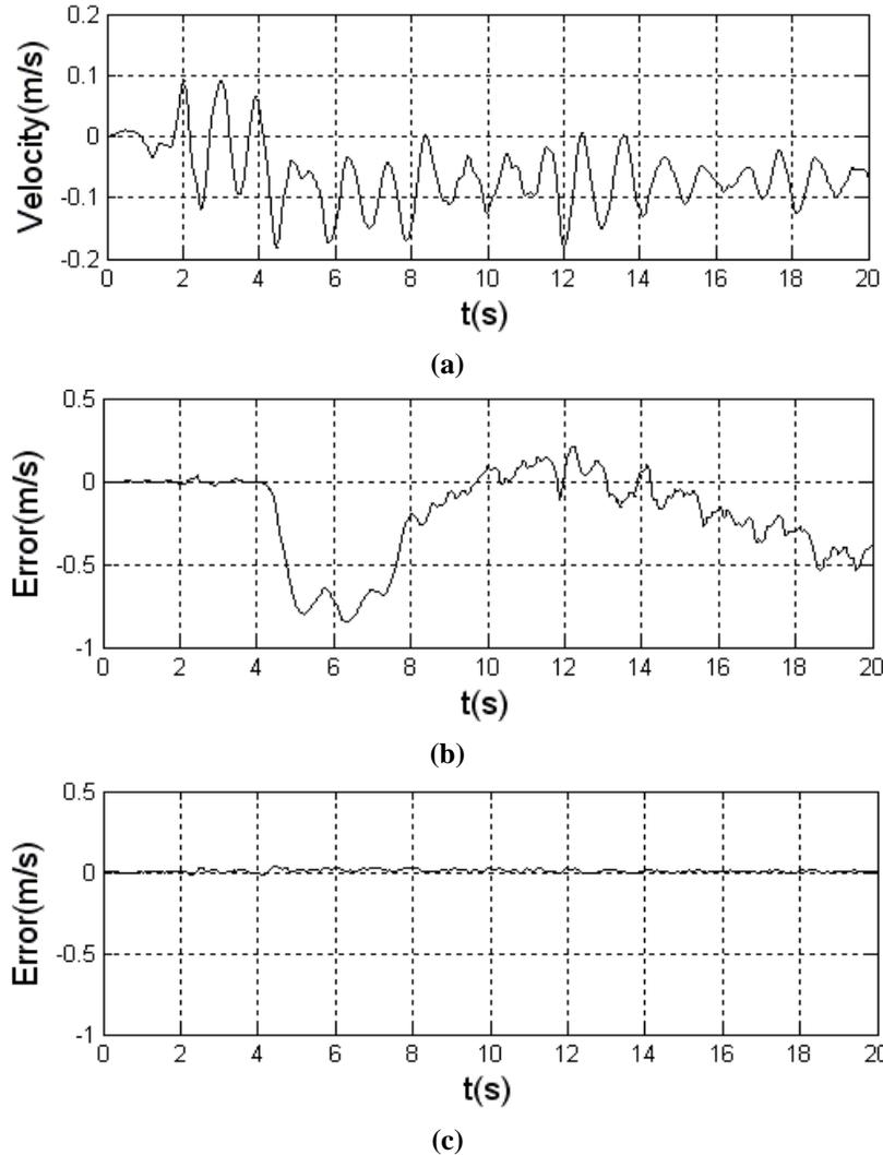
**Fig. 6.** Velocity of story 2 and estimated error under El Centro earthquake: a) velocity of story 2; b) estimated error of the first NN; c) estimated error of the second NN
