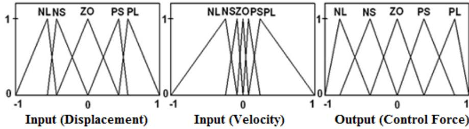
Fig. 3. Membership functions for inputs and output
