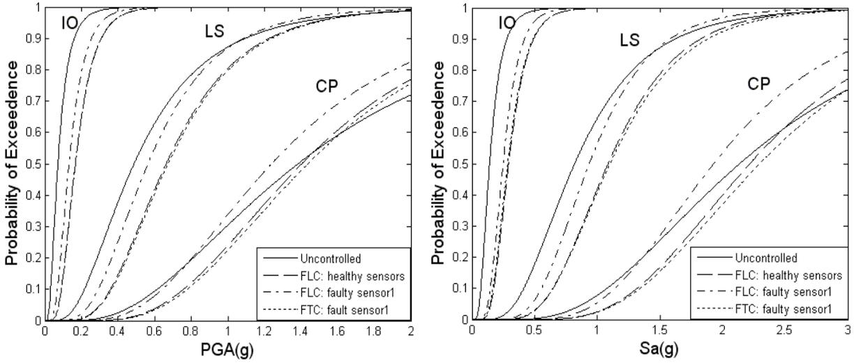
Fig. 7. Fragility curves for different controllers (fault can occur in sensor of story 1)
