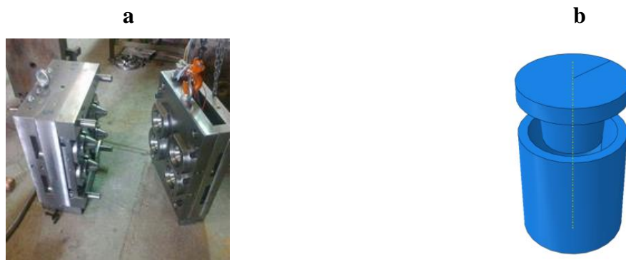
Figure 4. a) upper and lower jaws and b) punch and matrix modeling
