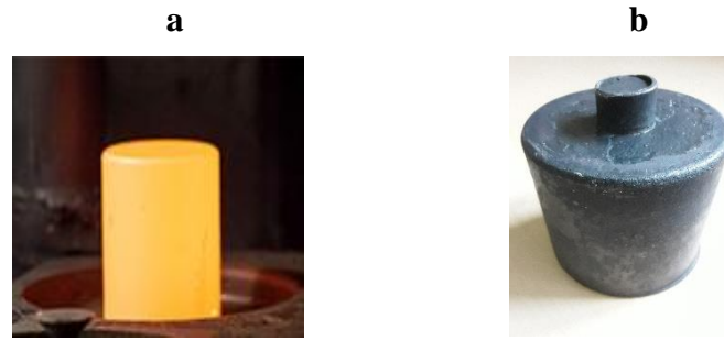
Figure 1. a) initial preheated and b) Final forged part
