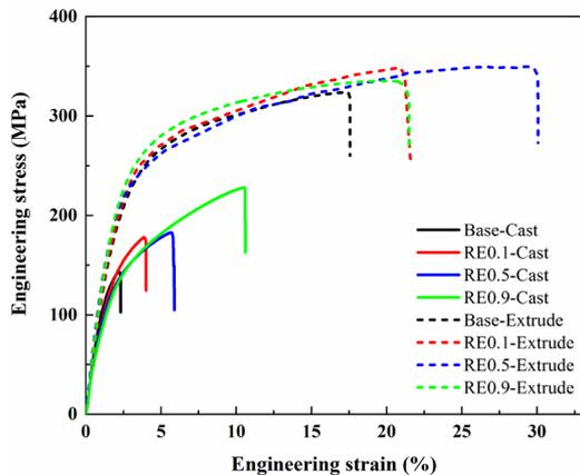
Fig. 3- Tensile stress-strain curves of the as-cast and as-extruded alloys.
