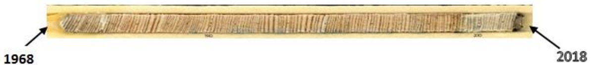
Fig. 3. Photograph of radial core showing the pith (year the tree was born, 1968) and the bark (year the tree was logged, 2018). The age of the tree is estimated to be 50 years.
