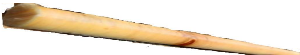
Fig. 2. Radial core of Swietenia mahogani obtained using increment tree borer.
