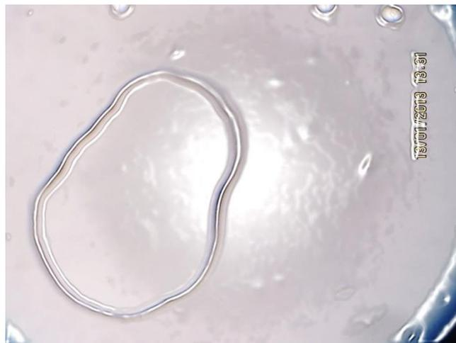
**Fig. 6.** Optical microscopy image of antifoam oil (500cP) with 10Mm size
