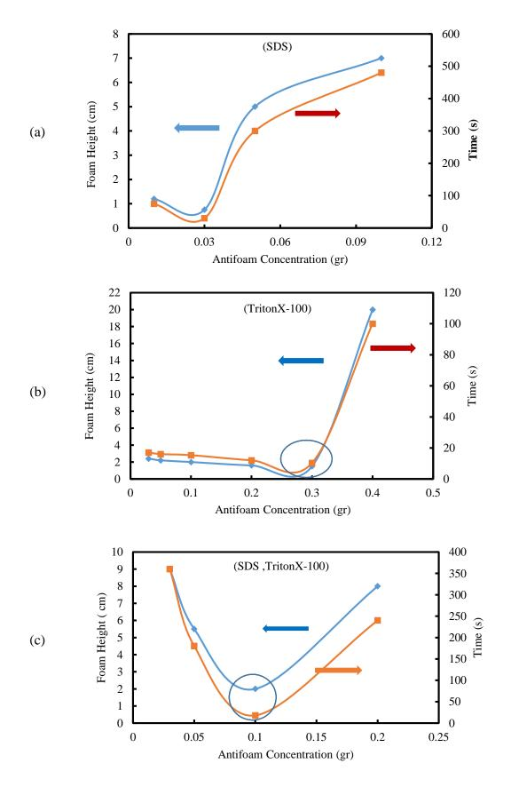
**Fig. 5**. The effect of different concentrations 0.01, 0.03, 0.05, 0.1 and 0.3g (a,b) 0.03,0.05,0.1,0.2,0.3 and 0.4 g oil viscosity, 500 cP (c) in both types surfactant solutions containing (0.02 g), anionic (SDS) and nonionic (Triton X-100)
