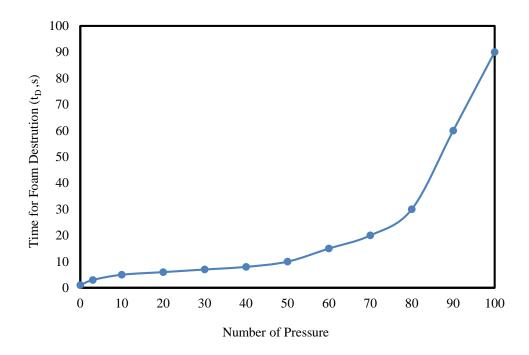
Fig. 8. Typical curve of exhaustion of antifoam in aqueous solution of 0.02 gr SDS
