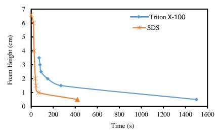
Fig. 2. Foam height with time for both surfactants. Triton X-100 (3.7 cm) SDS, (6.8 cm)
