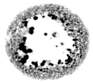
Fig. 4. View of antifoam lens sitting on surfactant solution (not visible). The dark objects are fluorescently labeled hydrophobic silica sitting on the aqueous-oil interface
