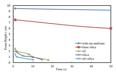
**Fig. 3.** Foam volume ( $V_F$ ) versus time (t) for antifoams by Bikerman test from a solution of the anionic surfactant Triton X-100 in the absence of antifoam and the presence of 0.1 gr of four different antifoams (a) fume silica (b) oil silicon (c) silica R794 (d) compound of silicone oil +hydrophobized silica particles
