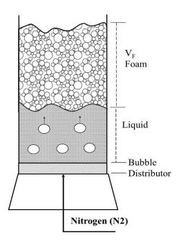
Fig. 1. Foam rise (bubbling) by the Bickerman method
