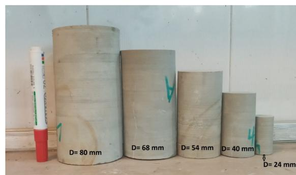
**Figure 5.** Core specimens at different diameters size (Sandstone 6)
