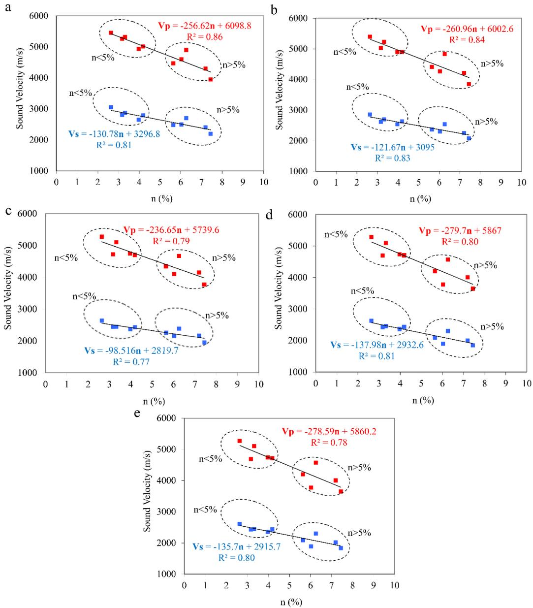
**Figure 11.** The correlation between Vp and Vs with n at different diameters size a: 24 mm, b: 40 mm, c: 54 mm, d: 68 mm, e: 80 mm
