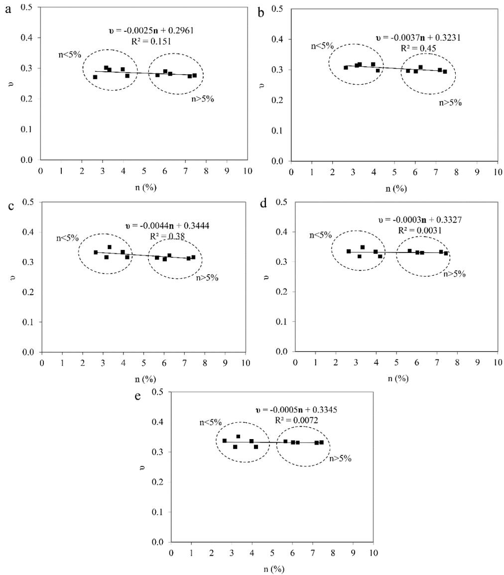
**Figure 13.** The correlation between  $v$  and  $n$  at different diameters size a: 24 mm, b: 40 mm, c: 54 mm, d: 68 mm, e: 80 mm
