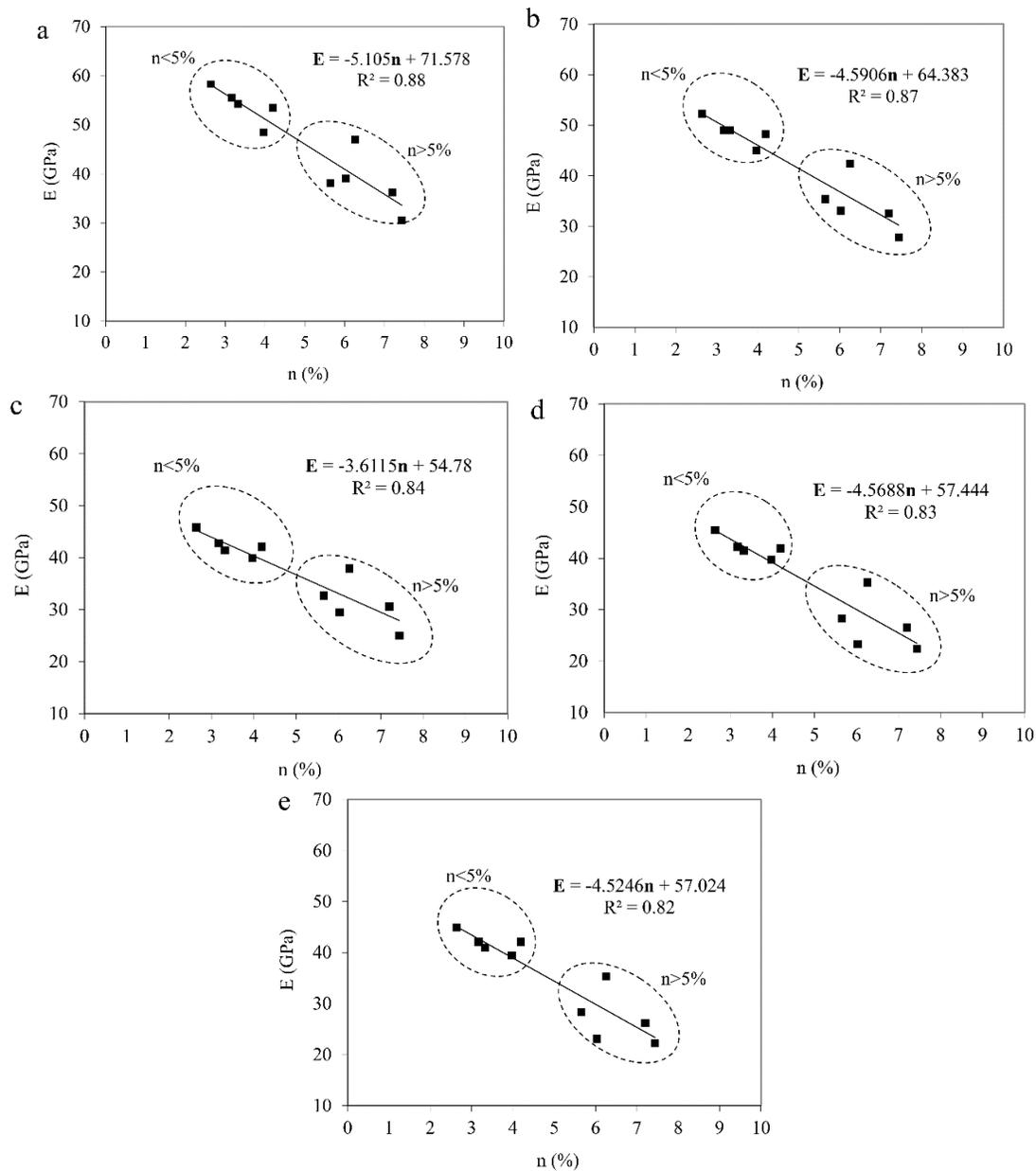
**Figure 12.** The correlation between E and n at different diameters size a: 24 mm, b: 40 mm, c: 54 mm, d: 68 mm, e: 80 mm
