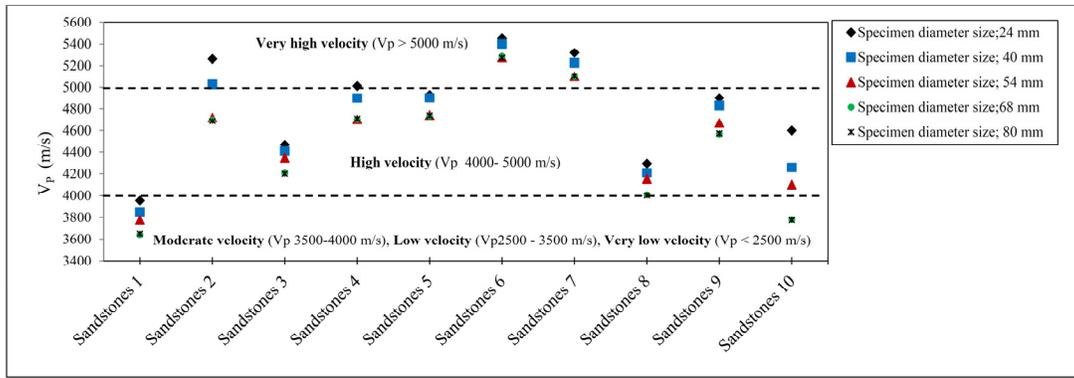
Figure 8. Classification of the sandstones based on  $V_p$  at different diameters size
