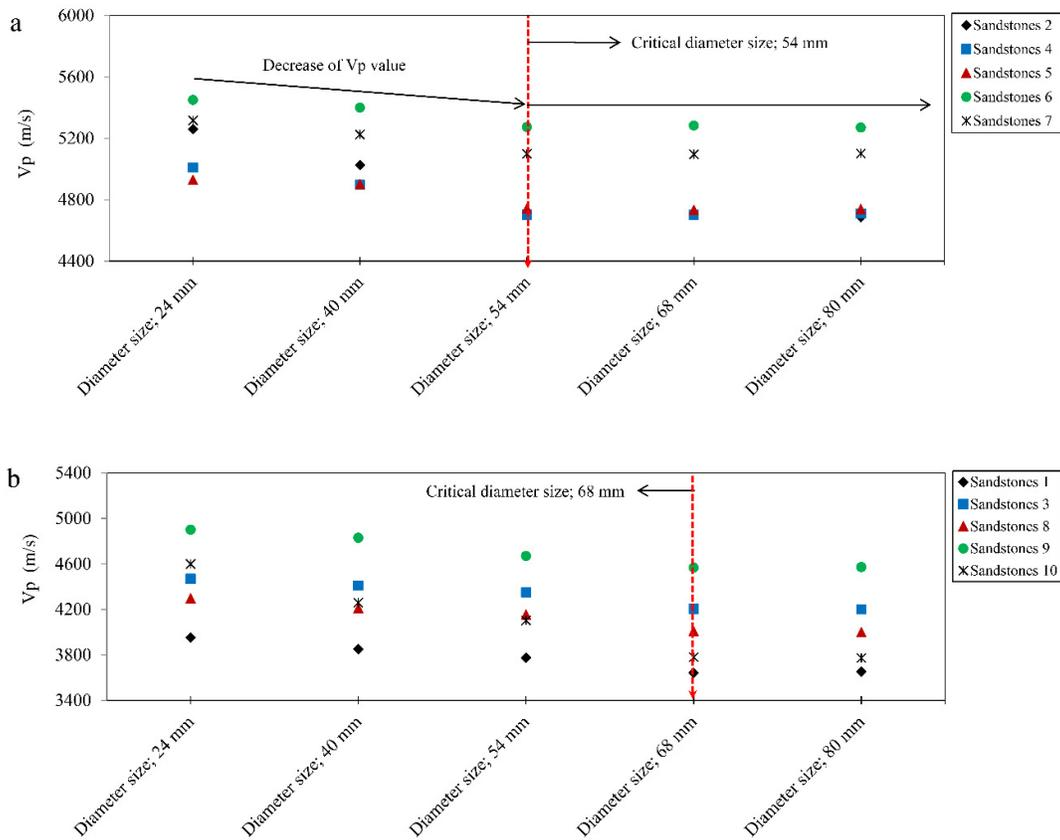
**Figure 6.** *V<sub>p</sub>* values of the sandstones at different diameters size a) Sandstones with porosity lower than 5% b) Sandstones with porosity higher than 5%
