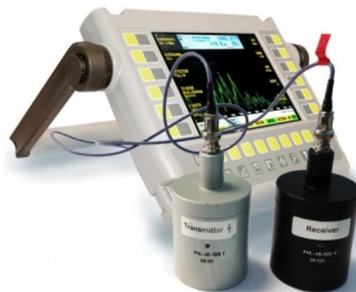
**Figure 4.** The ultrasonic pulse velocity testing equipment
