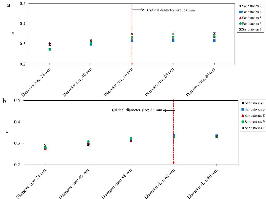
**Figure 10.**  $v$  values of the sandstones at different diameters size a) Sandstones with porosity lower than 5% b) Sandstones with porosity higher than 5%
