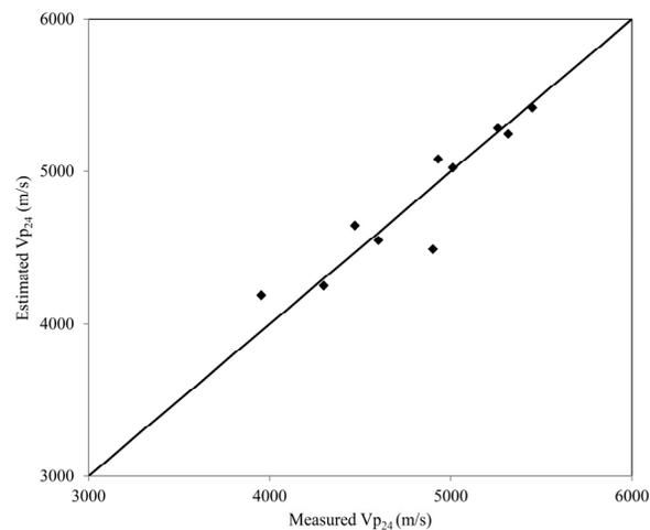
**Figure 14.** Measured  $V_p$  versus Estimated  $V_p$  from Eq. 5
