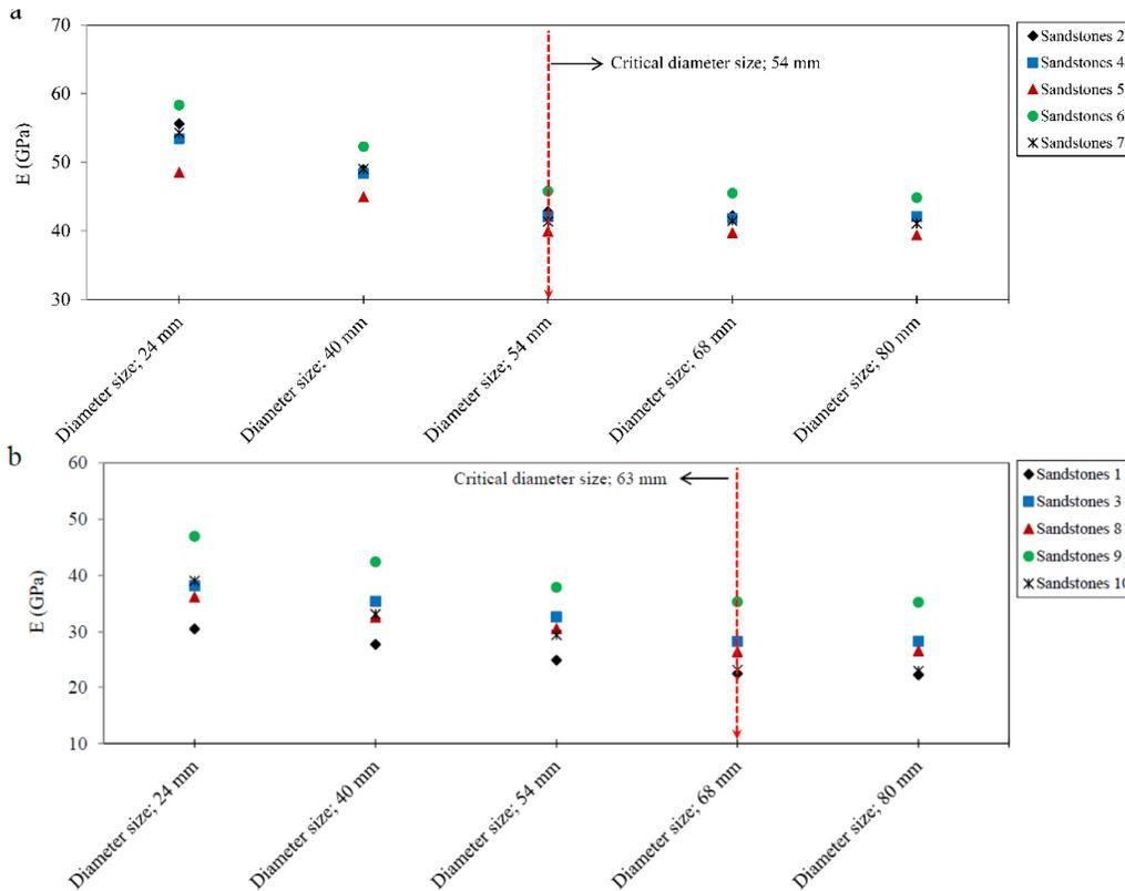
Figure 9. E values of the sandstones at different diameters size a) Sandstones with porosity lower than 5% b) Sandstones with porosity higher than 5%
