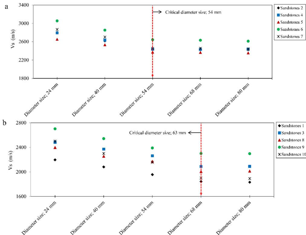
**Figure 7.**  $V_s$  values of the sandstones at different diameters size a) Sandstones with porosity lower than 5% b) Sandstones with porosity higher than 5%
