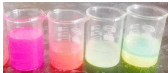
Figure 15. Photo-degradation of toxic azo dyes under UV irradiation with the aid of nanoparticles.
