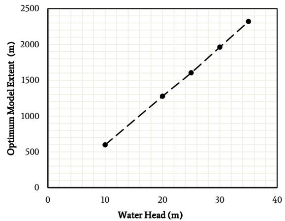
Fig. 10. The effect of water head on the optimal model extent.
