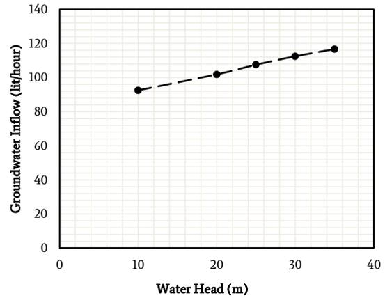
Fig. 9. The impact of water head values on the trend in groundwater inflow changes.
