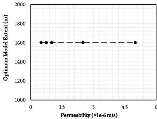
Fig. 8. The impact of the permeability coefficient on the numerical optimum model extent.
