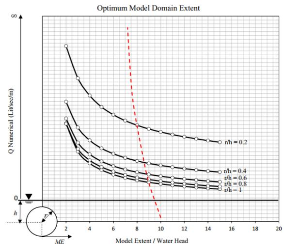
**Fig. 5.** A model is to determine the model domain extent. The chart shows the inflow rate ( $Q$ ) versus  $ME/h$  ( $ME$  model extent,  $h$  head) with different  $r/h$  ratios.
