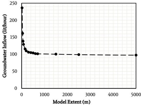
Fig. 6. The impact of model dimensions on the groundwater inflow rate.
