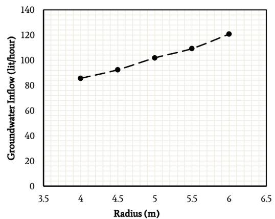
Fig. 11. The impact of tunnel radius on the groundwater inflow rate
