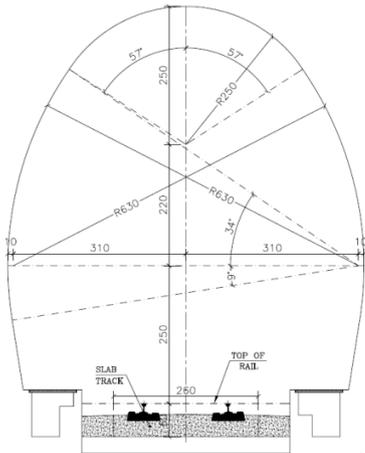
**Fig. 3.** The geometry and dimensions of the horseshoe cross-section for the km 78+493 tunnel.
