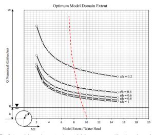
**Fig. 5**. A model is to determine the model domain extent. The chart shows the inflow rate (Q) versus ME/h (ME model extent, h head) with different r/h ratios. The red dashed line intersection with curves show the optimum model dimensions, which must be considered in producing the geological sections[26].
