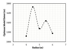
Fig. 12. The impact of tunnel radius on the optimal model extent.
