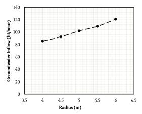
Fig. 11. The impact of tunnel radius on the groundwater inflow rate
