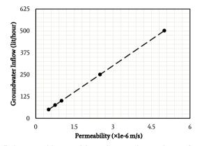
Fig. 7. The impact of the permeability coefficient on the groundwater inflow rate into the tunnel.
