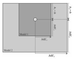
**Fig. 4.** Depth of model h and extend of model domain ME for two models with different ME, Subscripts refer to model 1 and model 2 [22].
