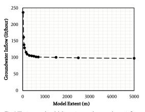
Fig. 6. The impact of model dimensions on the groundwater inflow rate.
