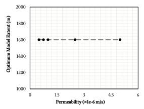
Fig. 8. The impact of the permeability coefficient on the numerical optimum model extent.
