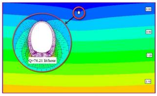
Fig. 13. Pore pressure contours in T<sup>b</sup> zone of tunnel.
