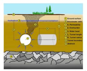
Fig. 2. Circular tunnel in a semi-infinite rock mass with a horizontal groundwater table [21].
