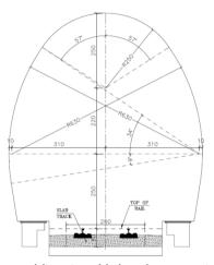
Fig. 3. The geometry and dimensions of the horseshoe cross-section for the km 78+493 tunnel.
