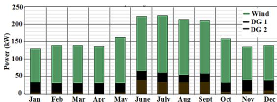
Figure 5. Monthly average power production of HRES installed in Zabol considering stable climate condition
