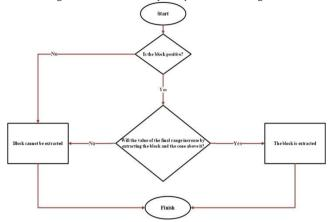
Figure 1: Decision making on extracting the block
