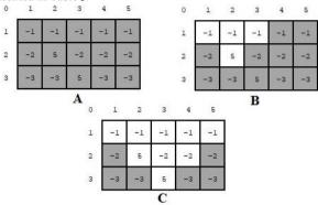
Figure 4: Formation of a larger cone with lower profit by floating cone algorithm
