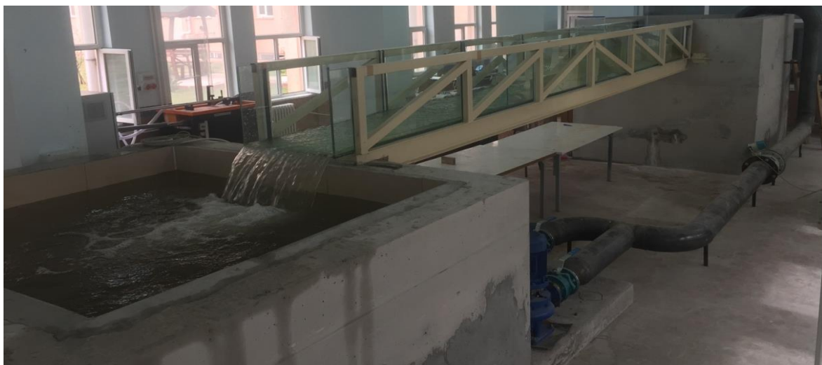
Figure 5. Open channel system used in experimental setup
