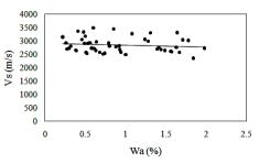
Fig. 6. The relationship between shear wave velocity and water absorption.
