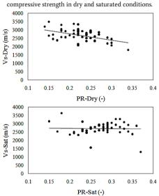
Fig. 11. The relationship between shear wave velocity and Poisson's ratio in dry and saturated conditions.
