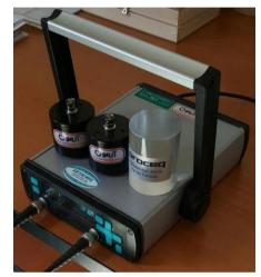
Fig. 4. The PUNDIT device used for  $V_{\text{s}}$  measurement.
