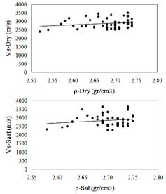
Fig. 5. The relationship between shear wave velocity and density in dry and saturated conditions.
