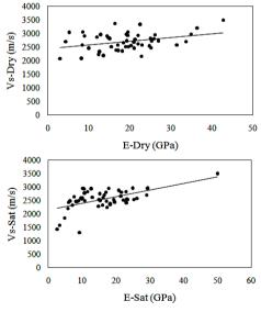
Fig. 9. The relationship between shear wave velocity and modulus of elasticity in dry and saturated conditions.
