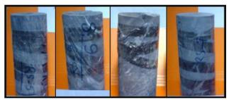
Fig. 3. The prepared core samples for conducting the laboratory tests.
