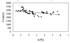
Fig. 7. The relationship between shear wave velocity and porosity.
